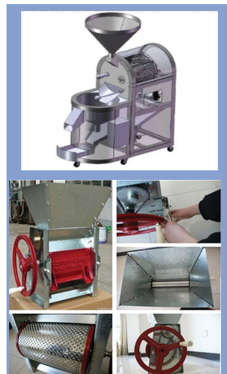
Figure 5. Sample pictures of the portable roasting and pulping machine being used in Region XI.
