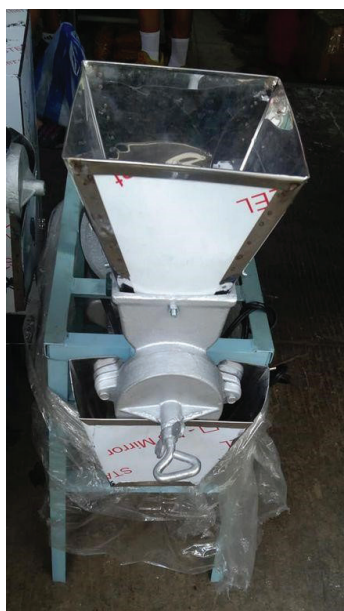
Figure 9. Sample picture of a locally fabricated peanut grinder.
