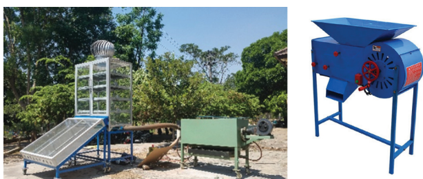
Figure 7. Coffee solar drying bed (L) and winnower (R) are other equipment that the farmers wish to be localized.
