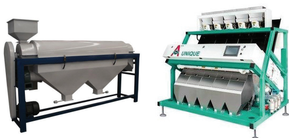
Figure 6. Imported coffee polishing machine (L) and coffee bean sorting machine (R) that the coffee farmers in Region VI wish to be localized.
