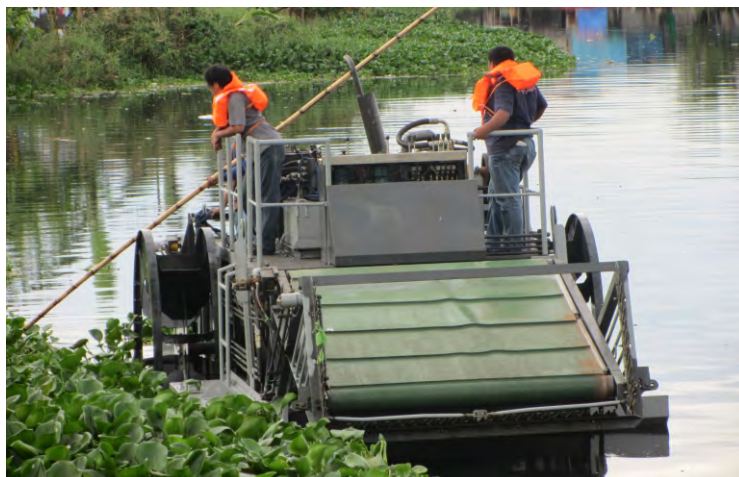
Water Hyacinth Harvester being tested at the Taguig portion of Laguna de Bay
