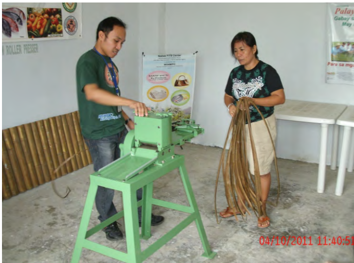
Engr. Allan John S. Limson of MIRDC (leftmost) demonstrates the use of the Pandanus Leaves Slitter-Presser machine
