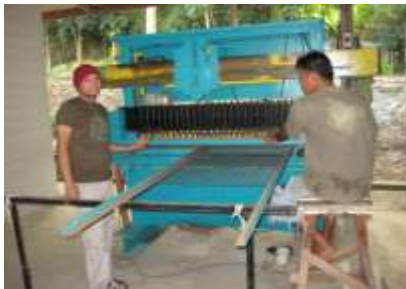
Multi-Spot Welding Machine being test run by MIRDC consultant for Egger Farm.
