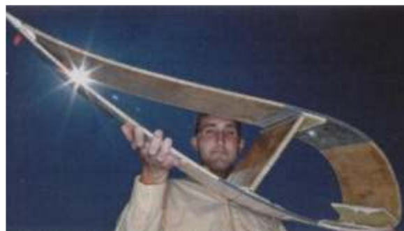
A cross section of a wind turbine blade like the one used in research to improve the efficiency of turbines and prevent damage to blades from high winds
