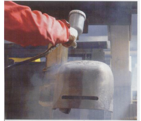
The innovative coating can be brushed or sprayed on
