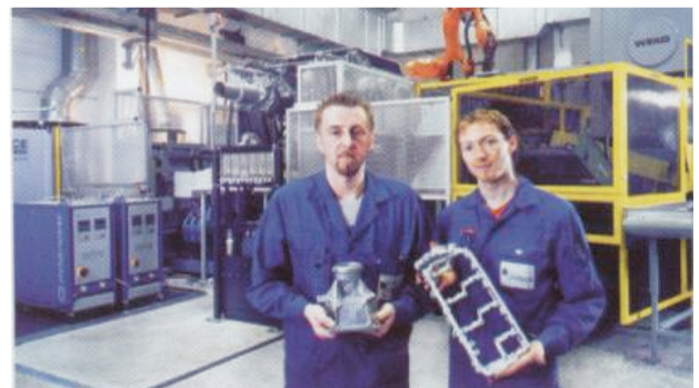
Two castings produced on the Carat die casting machine: holding device for a steering column (left) and cam carrier (right)
