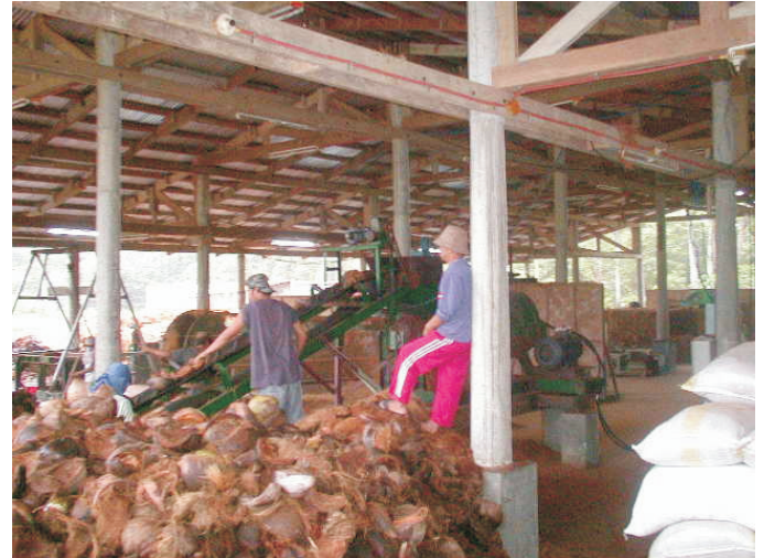
Enhancement of the Production Capacity of the Pilot Coco Coir Processing Center in Aurora Province - Retrofitting of the Decorticating Machine Conveying System
