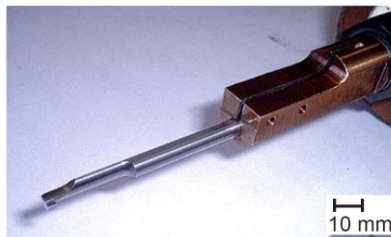
Figure 12. Non-rotational cutting tool used for 6-axis vibration cutting
