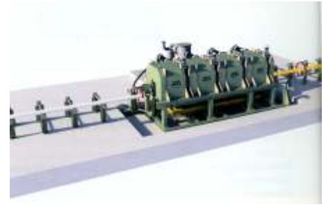
Line layout combining induction preheaters and heating furnaces.
