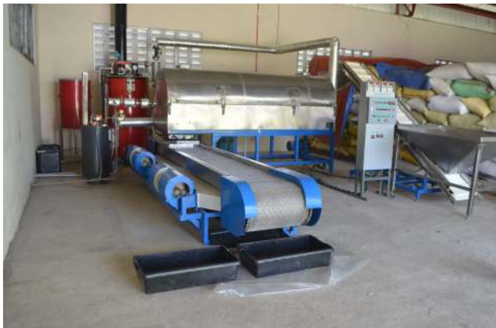
The developed Continuous-type Superheated Steam Treatment System for Stabilized Brown Rice.
