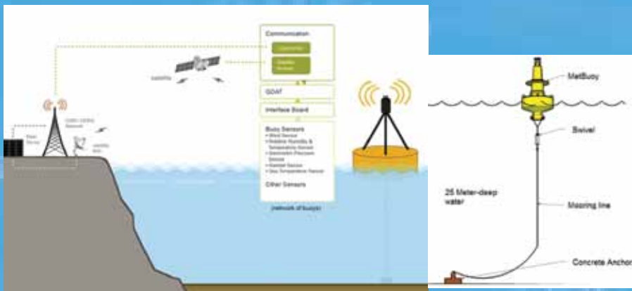
Communication of data from MetBuoy to ASTI server by satellite Schematic MetBuoy Assy. GSM networks.
