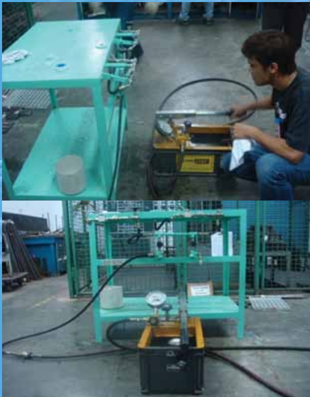
Figure 12. Actual hydrostatic testing of PSV Test Bench by one of the MML staff.
