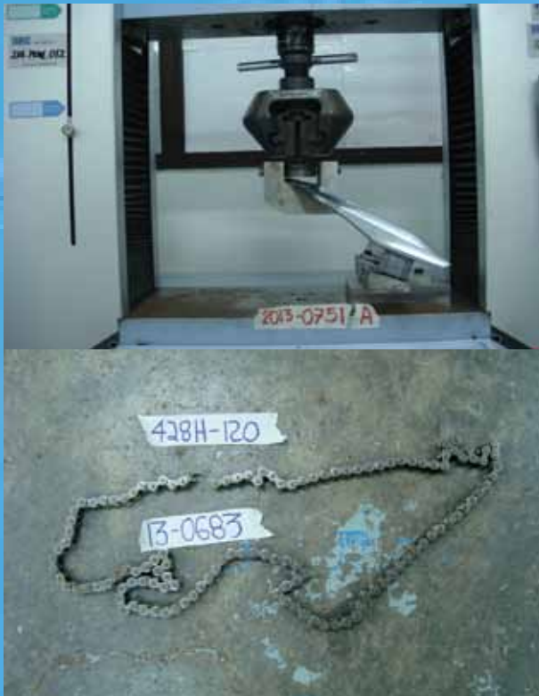
Figure 11. From top: Tension test of handle seat, and motorcycle roller chain for breakingload test.
