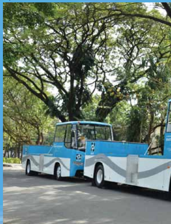
Figure 2. Actual Photograph of a 2-coach Prototype Hybrid Electric Road Train during a public demonstration at UP Diliman.
