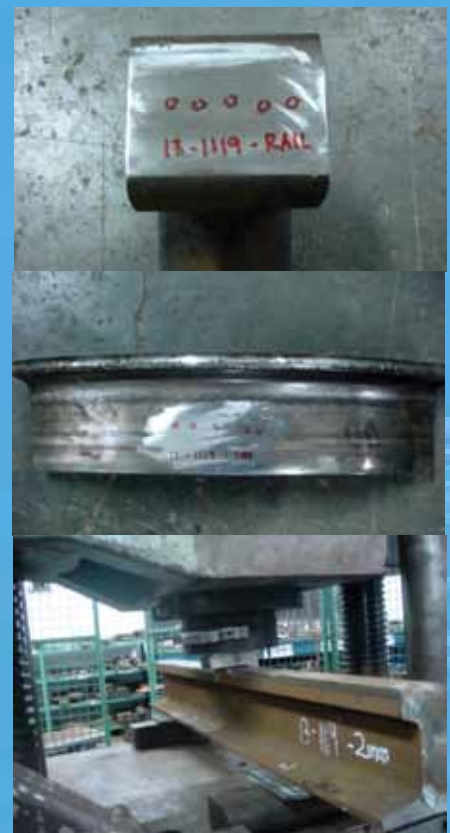
Figure 10. From top: Rail sample and wheel sample for hardness testing, and the actual compression testing of the sample using Universal Testing Machine (UTM).
