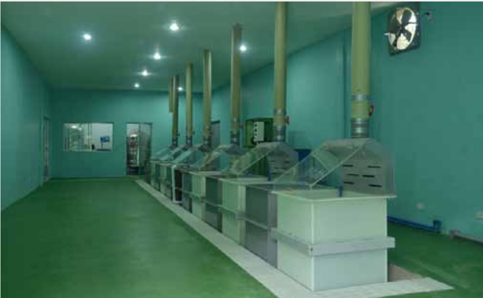
A complete line of anodizing process: cleaning, etching, desmutting, anodizing, dyeing, sealing and drying.
