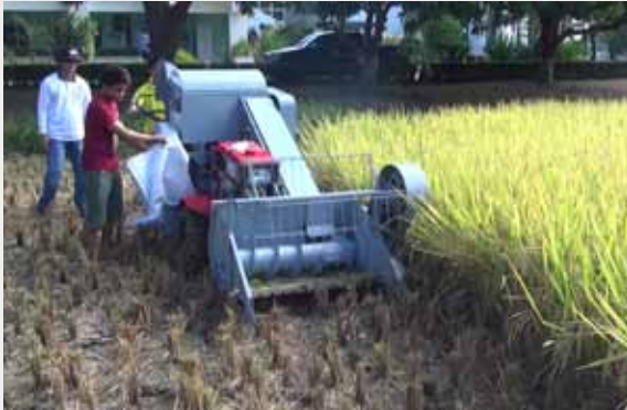
Functional testing of the hand tractor-attached harvester.
