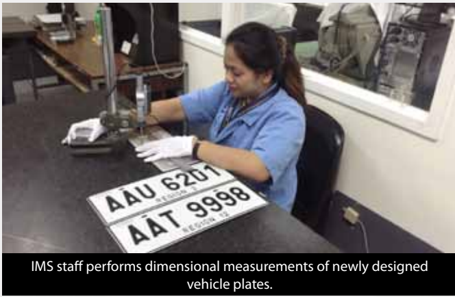
IMS checks the dimensional measurement of Business Plates submitted by NFA.
