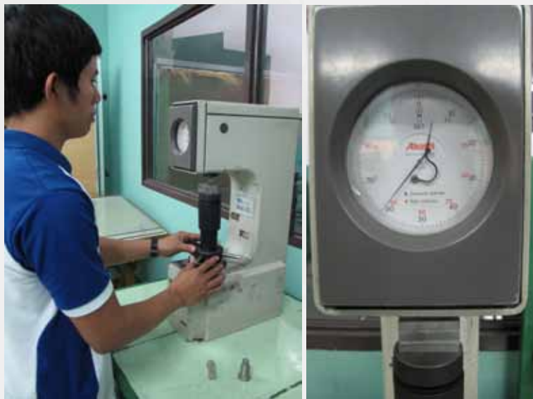
A HT personnel performs hardness testing on heat treated samples.
