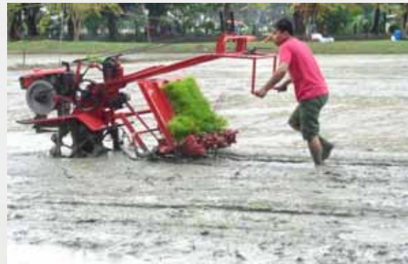
Field testing of the hand tractor-attached transplanter.
