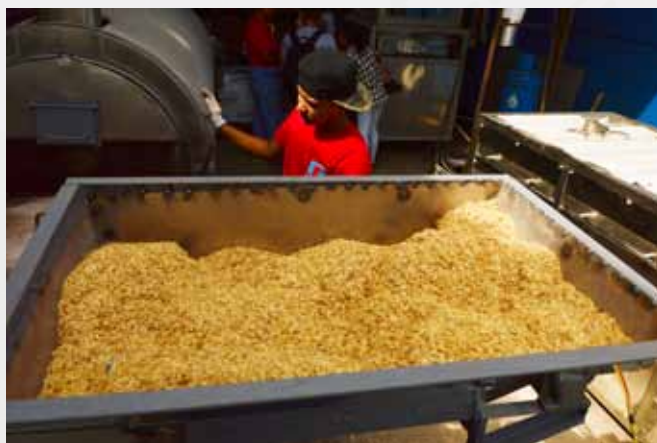
Rice hull as fuel source of the Fluidized Bed Dryer.
