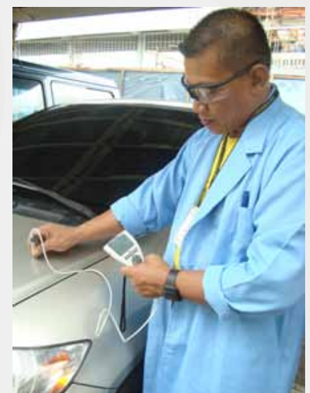
CLS personnel performs testing using portable thickness of coating tester .
