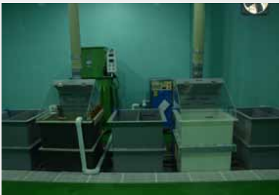
A rectifier is an electrical device used as a direct current power source to operate any plating or anodizing system.
