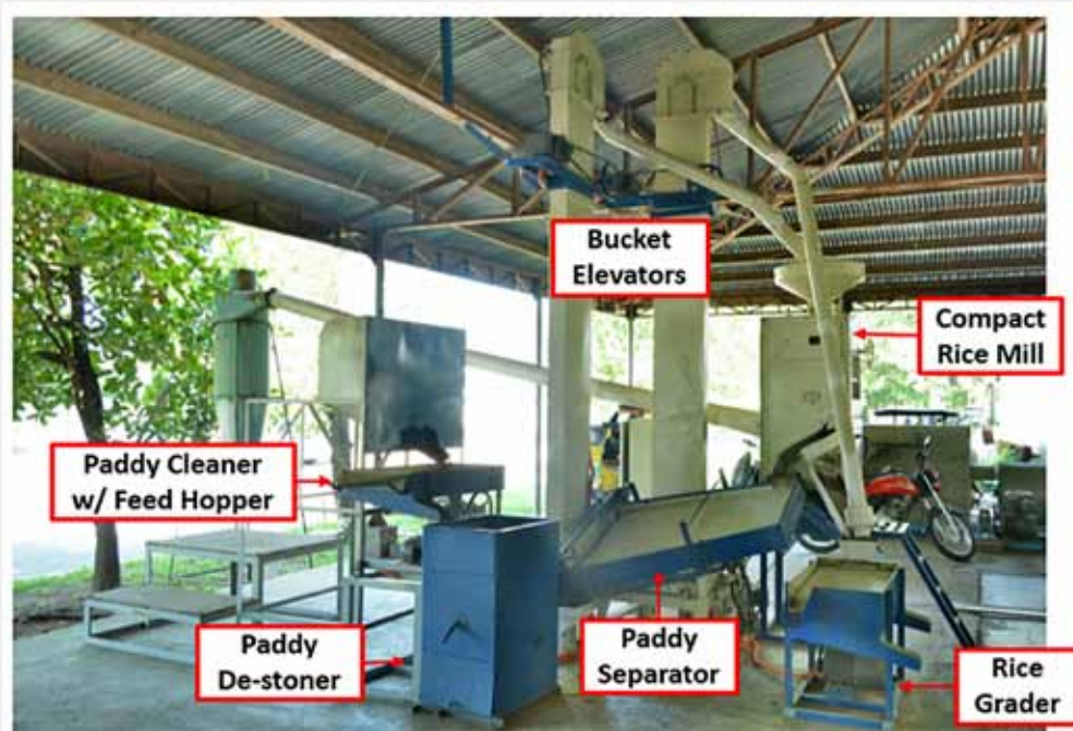
Complete set-up of a retrofitted compact rice mill system.
