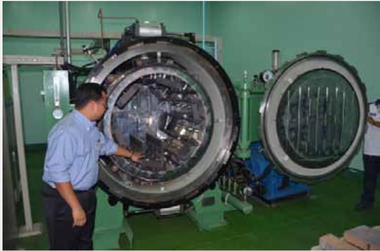
Engr. Nelson L. Tumibay explains the vacuum heat treatment furnace operations.
