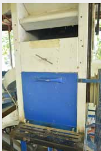
The diverting chute as attached to the compact rice mill.
