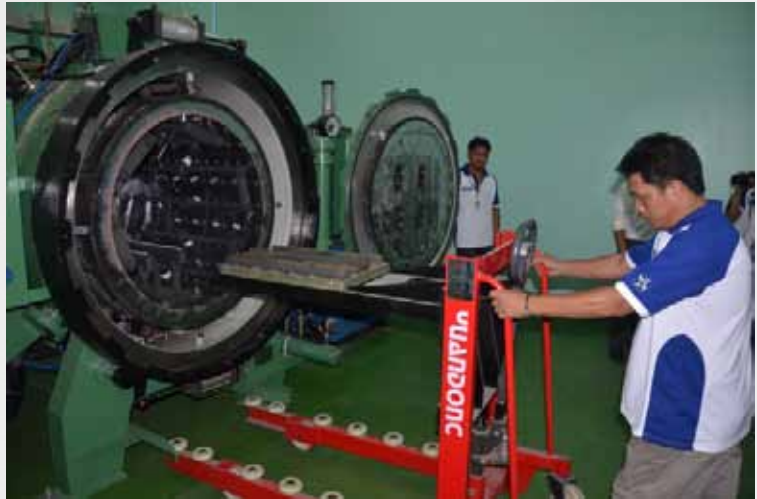
A technical staff charges D2 Tool Steels into the VHT Furnace for hardening heat treatment.
