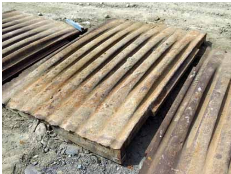
Worn-out austenitic manganese steel jaw crusher liner.
