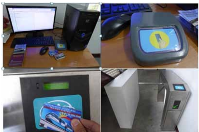
The Automated Fare Collection System consists of an AFC Software, smart card readers and automatic turnstile gates.
