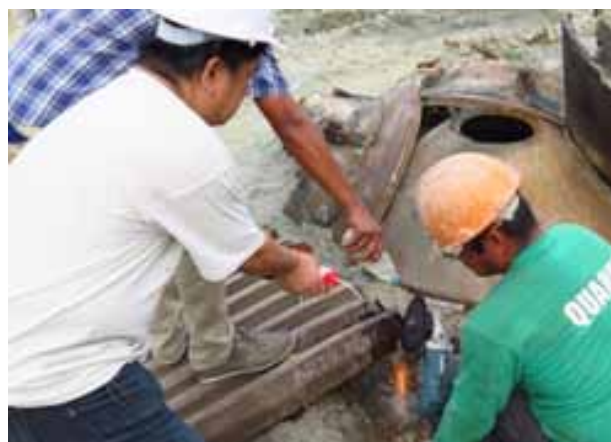
Cutting of sample from a jaw plate.
