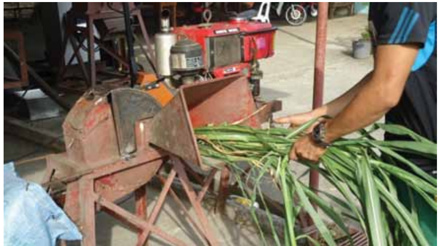
A side-cutting chopper with new blade under functional test .
