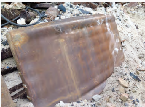
Fully worn-out jaw crusher liner. Achieving a fully worn-out jaw plate is one of the objectives of the AMS Project
