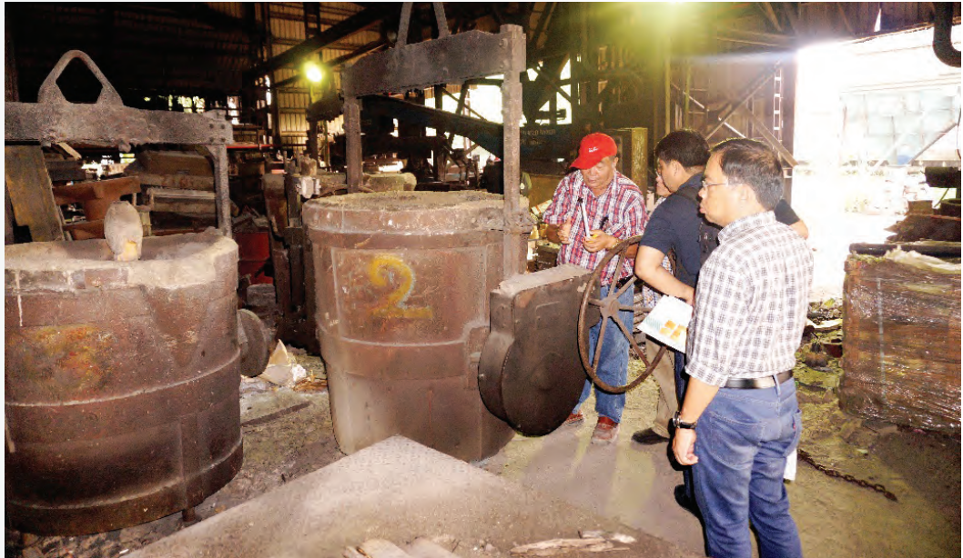
Bottom-pour ladles with different capacities at East Sun Steel and Iron.
