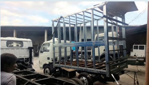
Structural design and fabrication of refrigerated container van
