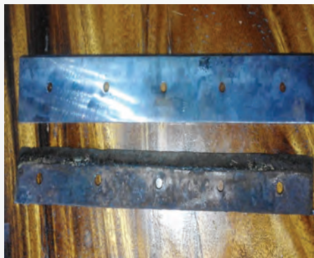
The new rotary blade (inverted) for the front cutting forage chopper and the replaced blade (bottom).
