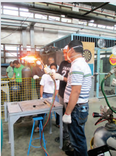
Engr. Dela Cruz shows the proper way to ignite and adjust a brazing flame.
