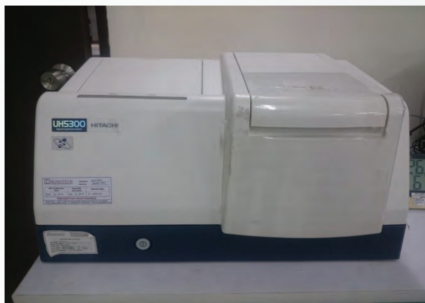
Hitachi UH-5300 UV-Vis Spectrophotometer (used for the analysis of Phosphorus and Molybdenum)
