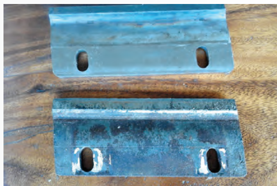
(Center picture) The old (top) and new (bottom) rotary blades. (Right picture) The stationary blades, new (left) and the original (right).
