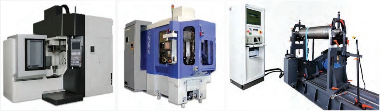
Newly acquired equipment (from left): 5-Axis CNC Machine Okuma MU6300V, Gear Hobbing Machine GE25A, and Dynamic Balancer CMAT CMT 1500.
