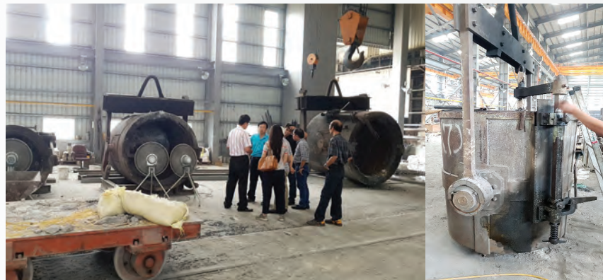
Bottom-pour ladle at Hong Shing Foundry.
