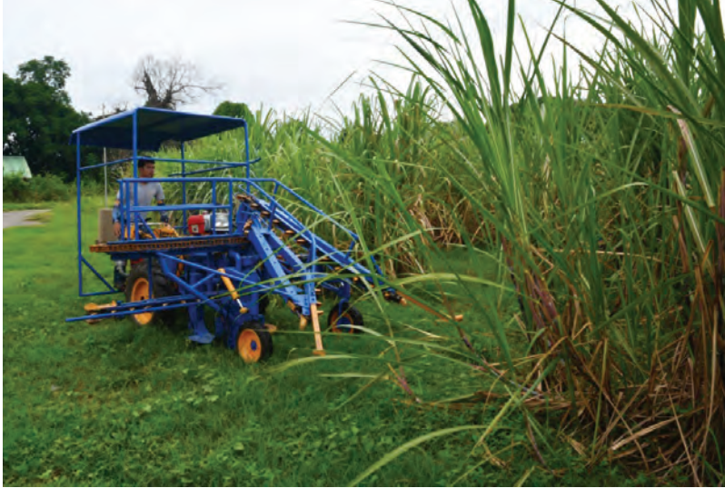
Functional Testing of Sugarcane Cutter.
