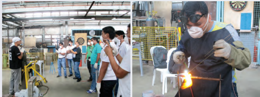
(L) Engr. Reynaldo L. Dela Cruz Jr. demonstrates proper handling and set-up of cylinders, (R) A Brazing Processes participant performs actual brazing on copper tubings.
