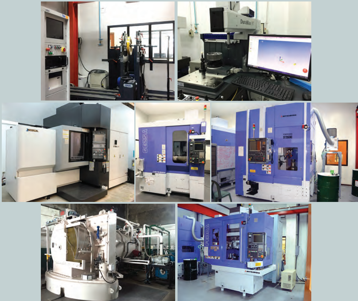
Newly acquired equipment (from left): Gear Measuring Equipment, Dynamic Balancer CIMAT-1500 H2P, CNC 5-axis Vertical Machining Center Okuma MU-6300V, CNC Gear Hobbing Machine GE25A, CNC Gear Shaping Machine ST25CNC, Vacuum Carburizing Machine and CNC Gear Shaving Machine FE30A
