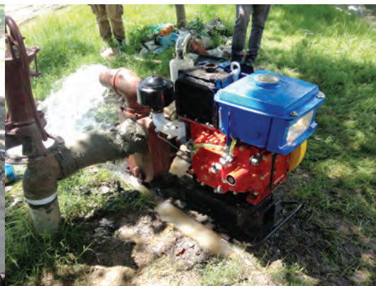
Field testing of prototype coupled to a 3"x3" water pump dryer
