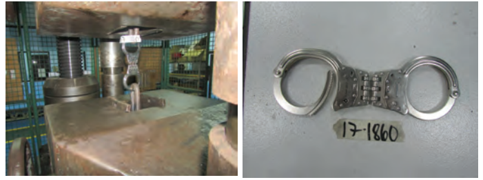
MIRDC tests handcuff sample to determine the strength of the new design
