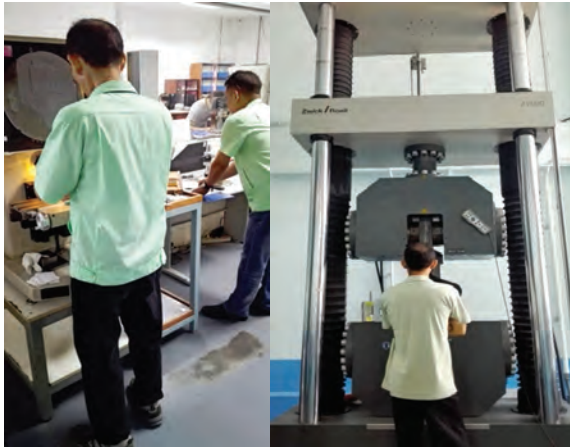
Experienced technicians from the Metrology Laboratory of the Instrumentation and Metrology Section perform calibration inside the laboratory (left) and in the field (right).
