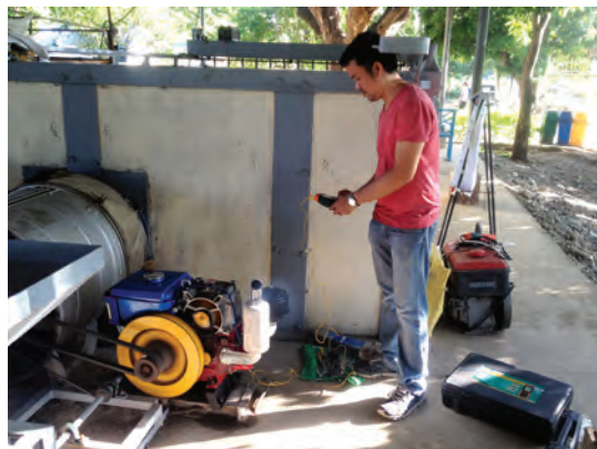
Field Testing of Prototype Coupled to a 5-ton capacity flatbed dryer
