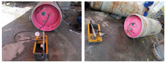
Sample refrigerant tanks tested for leaks
