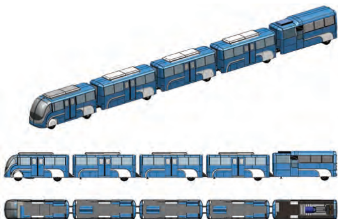
(Left) Proposed commercial model of the Hybrid Electric Road Train with a rounder face of the Pilot Coach. (Right) The new configuration of the motors in the commercial model of the HERT. Instead of the previous vertical configuration, the motor will be horizontally placed under the chassis to accommodate more passengers inside the coaches
