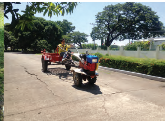
Field testing of prototype coupled to an agricultural trailer
