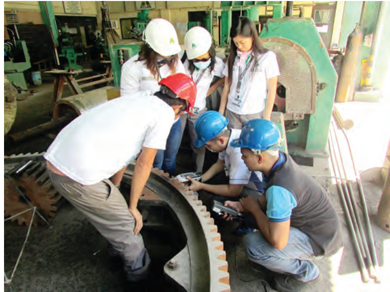
PCL staff conduct on-site chemical analysis on gears used by a fertilizer company in Cebu.
