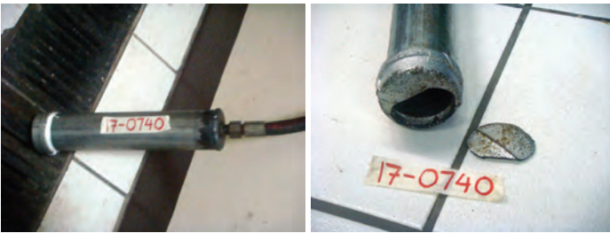
Steel pipe brought by the PNP ordinance group to determine their pressure capacity
