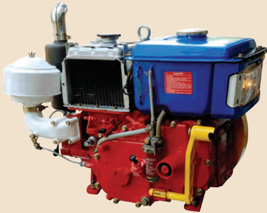
12hp Single Cylinder Diesel Engine Prototype
