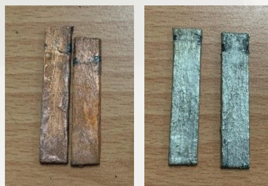
Carbon conductive paint electroplated with copper (left) and nickel (right).
