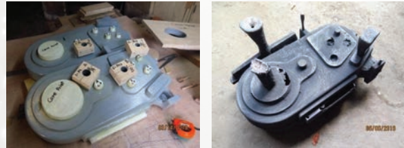
(Left) Wood patterns for the gearbox housing; (Right) As cast gearbox housing
