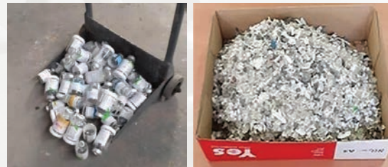
Sample medical vials before and after crushing
