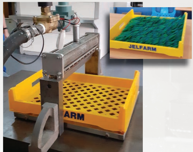
Test rig for drying; Pallet full of okra for drying (inset).
