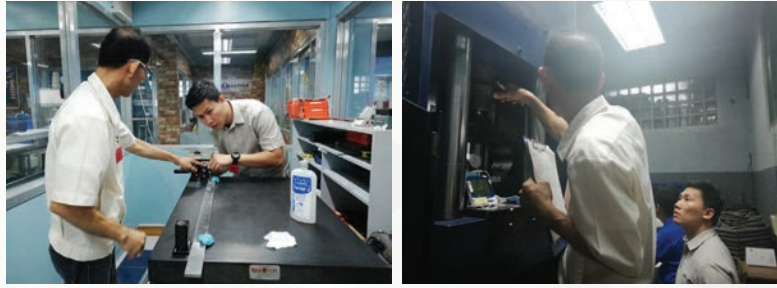
The Metrology Laboratory staff conduct onsite calibration of granite plate (left) and UTM (right).
