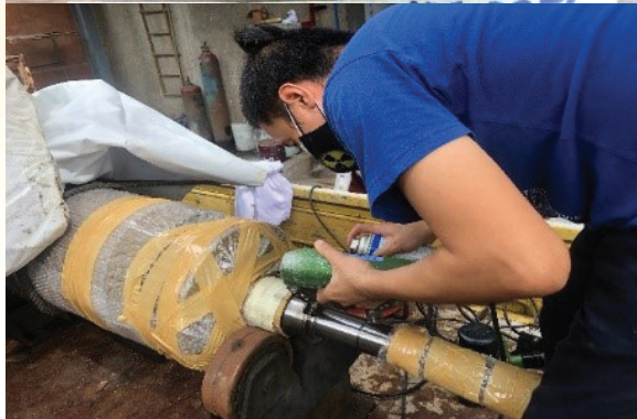
Bond Test on Babbitt Bushing and Magnetic Particle Testing and Ultrasonic Testing of Shaft
