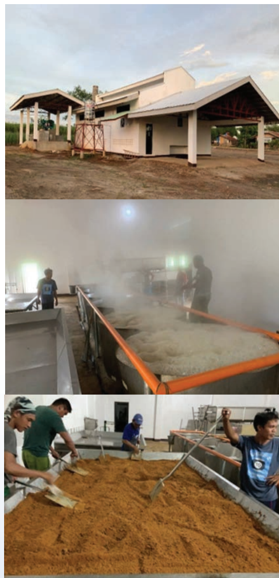
Figure 4. (From top) Boling, Milling & Bagasse Houses; Evaporator Sets (Cooking Vats); and Cooling Rough.
