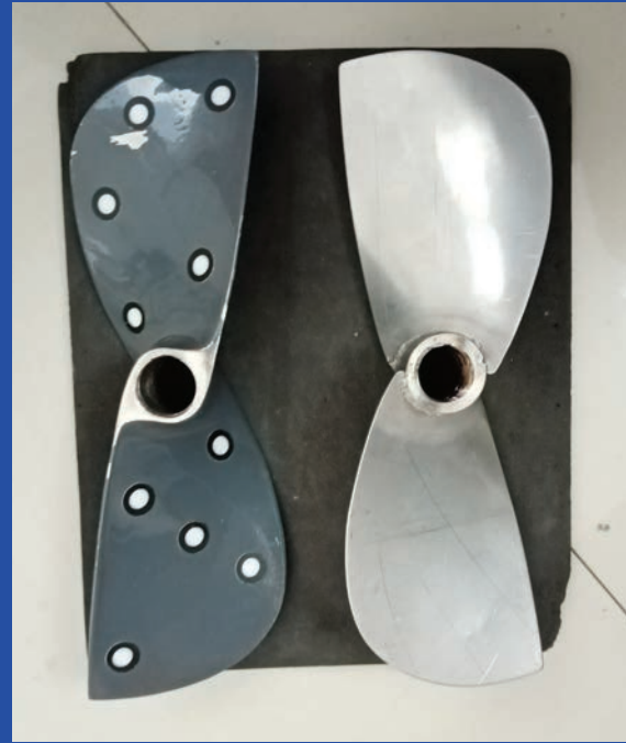
Aton Marketing's SS impeller blade (left) and SS impeller blade produced using the alternative process (right)
