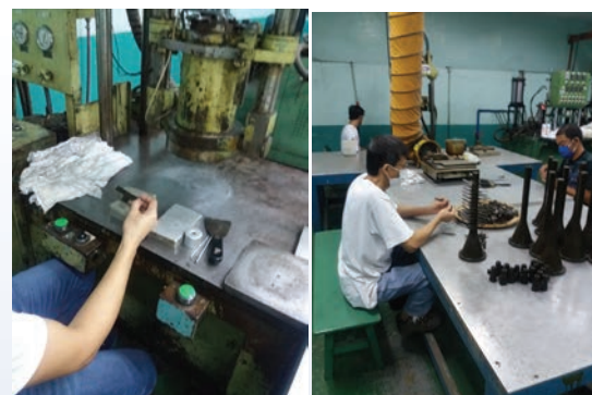
(L) Wax molds being repaired, cleaned and prepared for ceramic coating (R) Wax injection machine on the job producing wax items for investment casting process.
