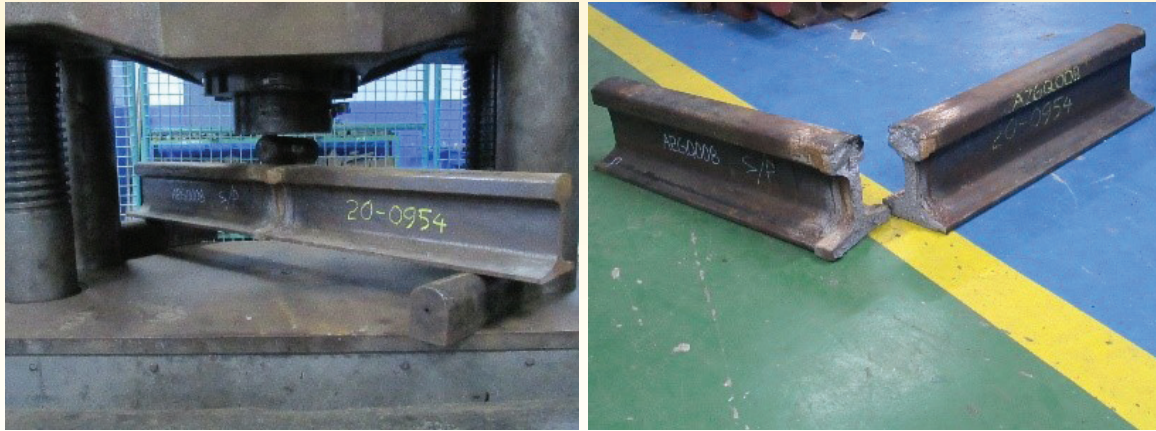
Before and after the application of flexure load on Thermit welded rails
