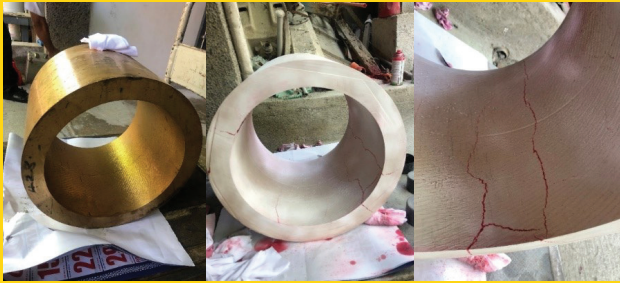
Defect on Tiger Bronze Bushing after the conduct of PT
