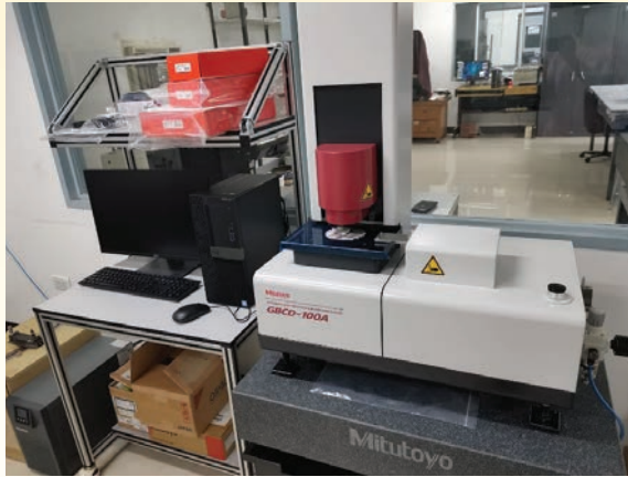
(L) New Comparator GBCD-100A that can calibrate grade 0 steel and ceramic up to 0-100mm; (R) Dimensional measurement of test sieve
