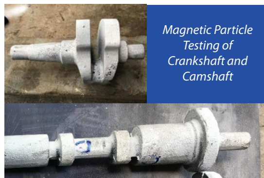
Bond Test on Babbitt Bushing and Magnetic Particle Testing and Ultrasonic Testing of Shaft
