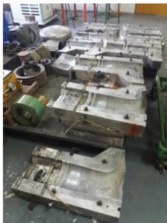
Ready for delivery: Laser-welded aluminum molds of boots with new logos
