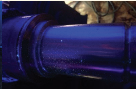
Bond Test on Babbitt Bushing and Magnetic Particle Testing and Ultrasonic Testing of Shaft
