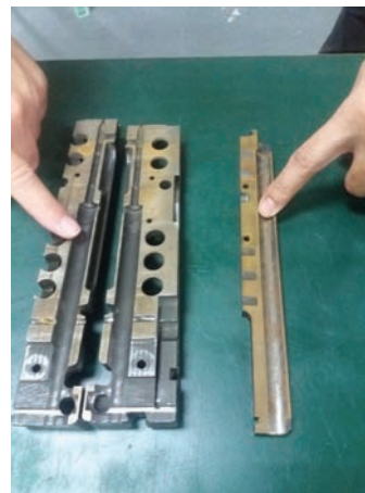
50 caliber machine gun bolt wire cut for measurement insert and CAD CAM programming
