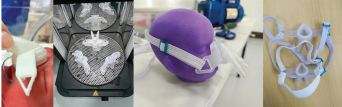
(Left to Right) Initial design test fitting, revised design, revised design test fitting, nasal mask assembly.
