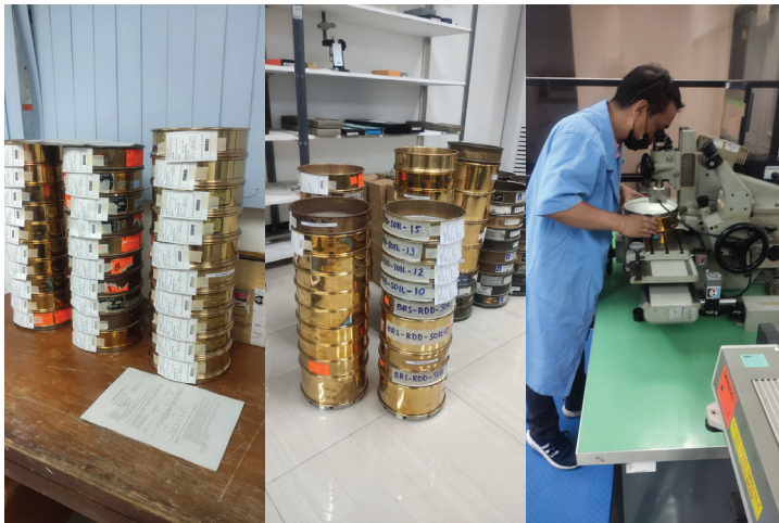
Dimensional measurement of test sieves with the Metrology Laboratory's New Comparator GBCD-100A that can calibrate grade 0 steel and ceramic up to 0-100mm.
