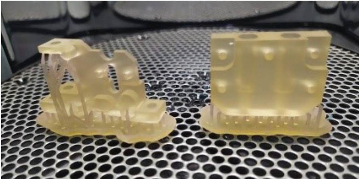
High-temperature plastic satellite components manufactured via SLA.
