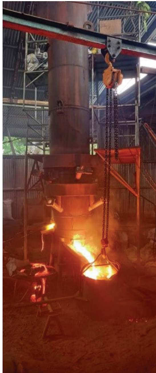
Actual operation of improved MPEW Cupola Furnace.
