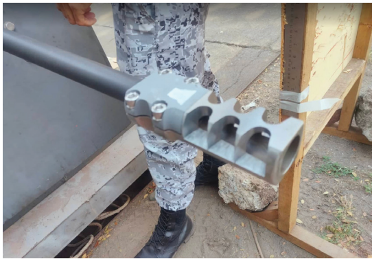
The locally-fabricated compensator prototype.
