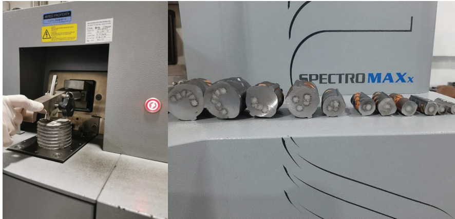
Testing of hexagonal bolts and deformed bars by the ATD's Physico-Chemical Laboratory and Corrosion Laboratory under Analytical Laboratories Section (ALS) supervised by Engr. Gina A. Catalan for the "Build, Build, Build" program of the government.
