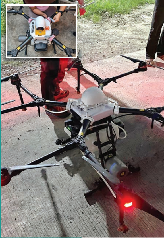
The 3D-printed drone attachments which uses fewer materials without compromising its mechanical integrity.
