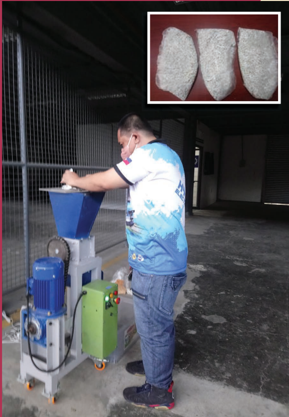
The improved plastic shredder which can process ASA plastic.
