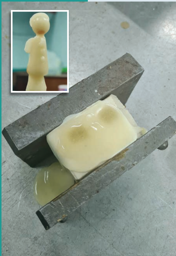
A photo of the improved pattern wax material made of locally available materials.
