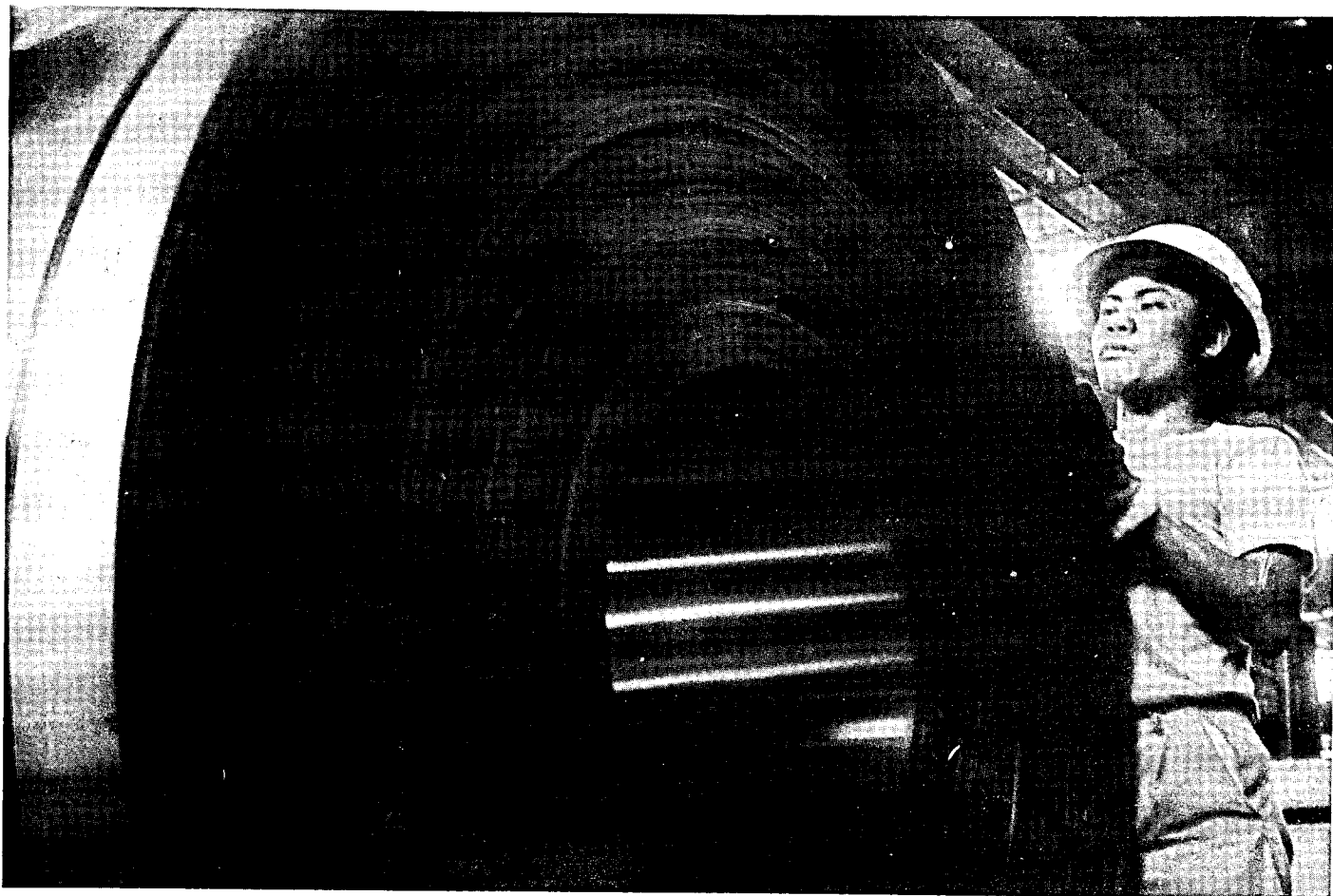
An annealed coil is being checked by an operator, prior to processing at ELIROL's Temper Mill for the desired hardness.
