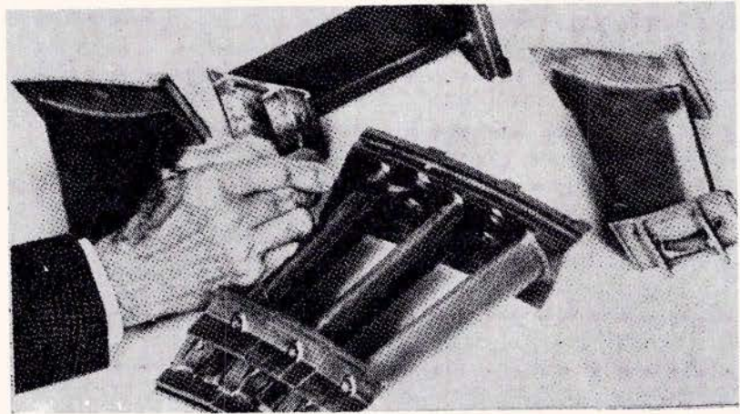
This fabricated jet engine turbine nozzle assembly demonstrates the capability of the activated diffusion bonding process. The three vanes are joined at both the inner and outer bands.
