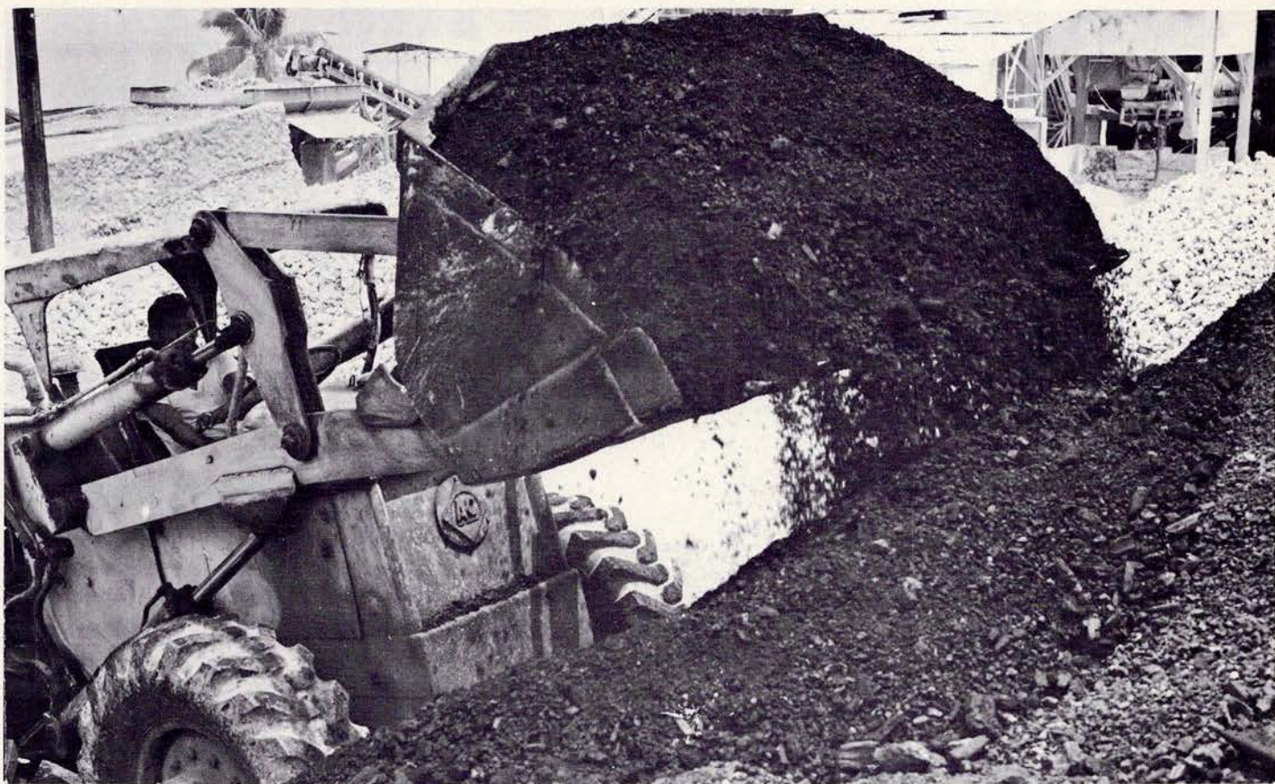
Charcoal is an ingredient in both calcium carbide and ferro alloy manufacture.
