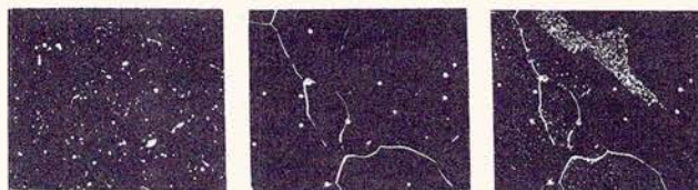
Carbon steel with 0.2% C \alpha - \gamma transformation Incident-light dark-ground 200X
