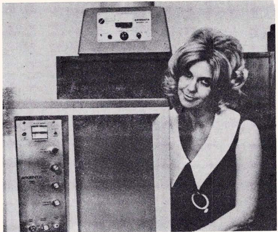
Compact "Argenta" electrolytic silver recovery unit can be distaff operated. Two new models are shown here.
