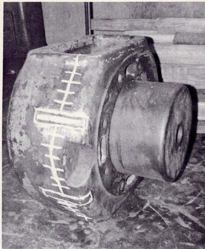
The repaired compressor.
