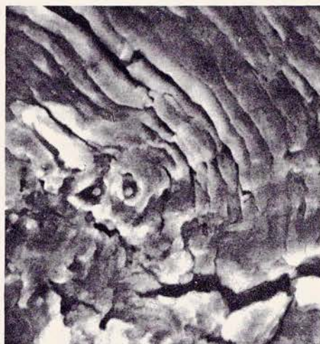
Striations on a mild steel fatigue surface. Magnification, 2700 times.
