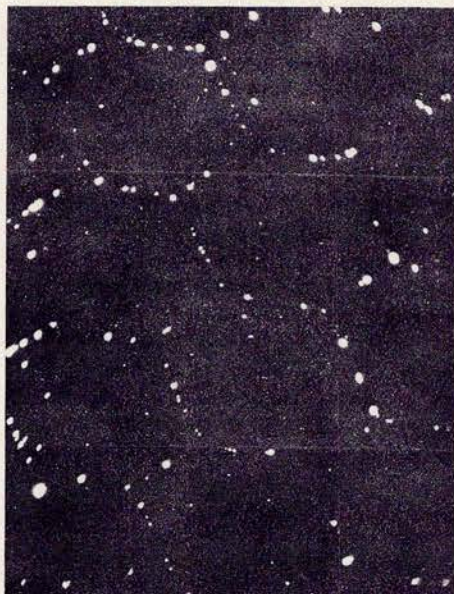
Decanted solid; liquid interface of an aluminum crystal exhibiting cellular growth, showing pores in cell walls after electroplating. Magnification 272 times.
