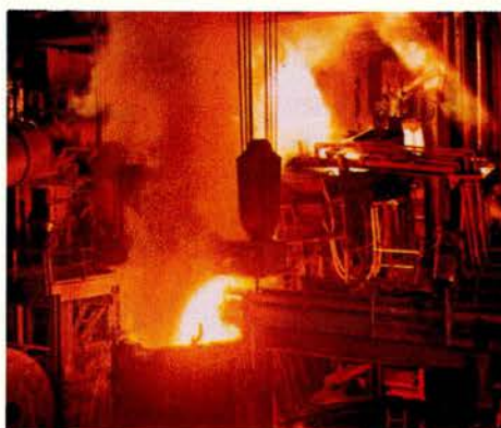
Tapping an arc furnace.
