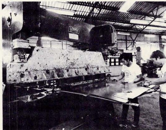
The foodliner of a refrigerator in its flat sheet form are press worked in the 40-ton press brake.
