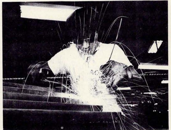
Gaps at the corner of door panels are closed by brazing.
