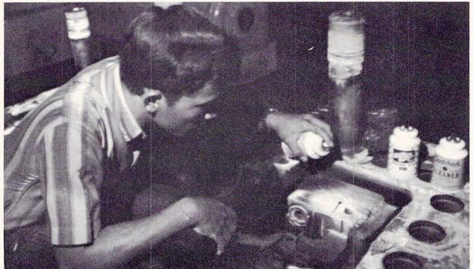
Dye penetrant testing of a turbine diaphragm.
