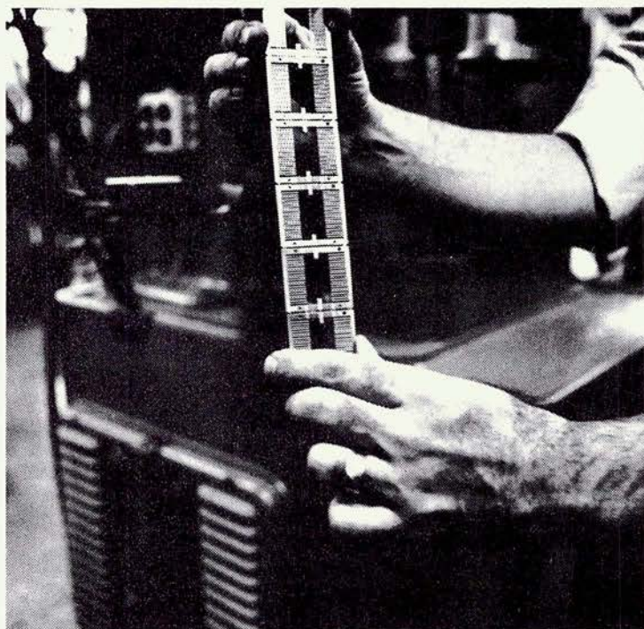
Tolerances on gold-striped strip stampings for electronic devices are held to as close as 50 millionths of inch thickness.
