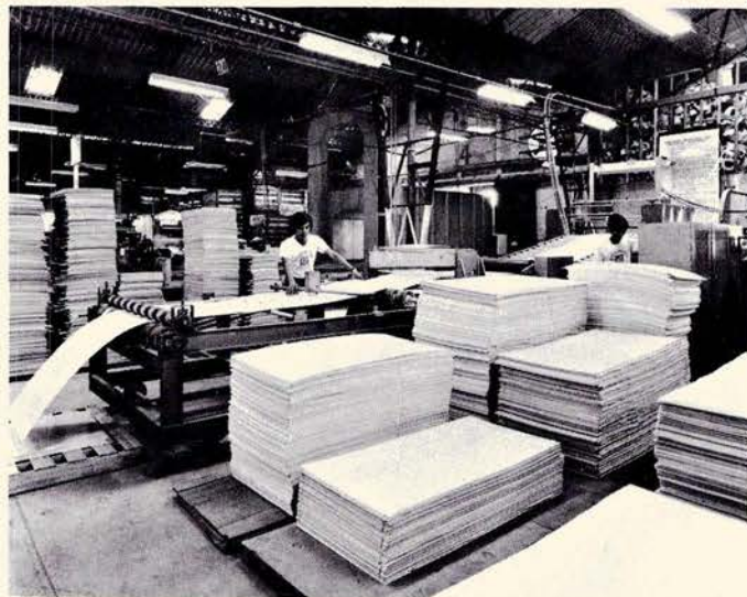
Plastic sheets from the extruder undergoing rolling and shearing processes.
