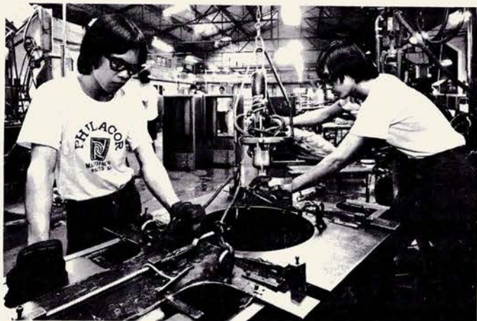
A refrigerator cabinet being assembled by spotwelding.
