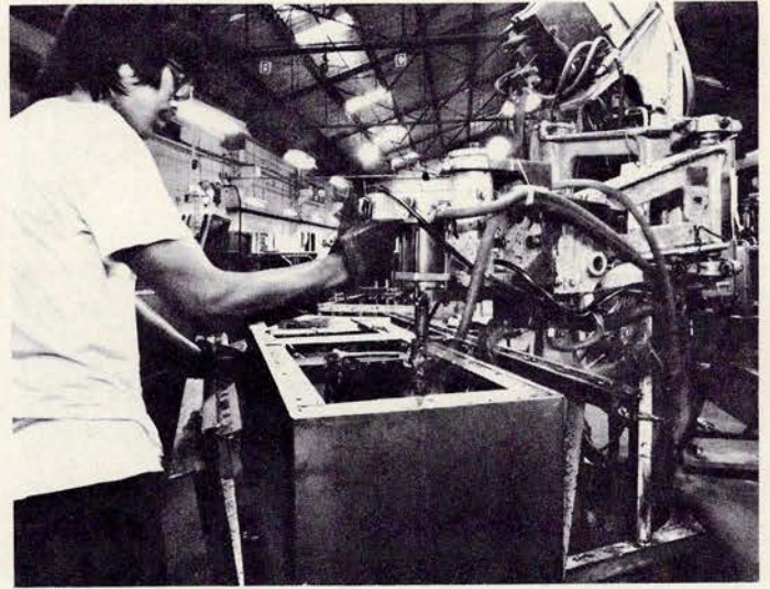
A 75-KVA spotwelder used in spot welding the rear panels to the refrigerator cabinet.
