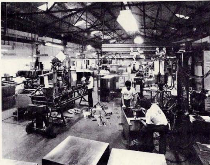
A partial view of the Weld Shop, where finished metal parts are assembled into desired structure using jigs and fixtures as guides.
