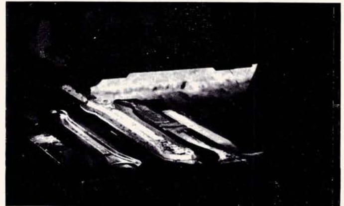
After heating to a plastic state, blanks are forged in drop forge hammers.
