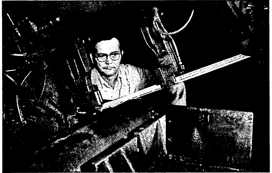
Effectiveness of welds on the high speed band saw blade is being checked after production by new welding and annealing method.
