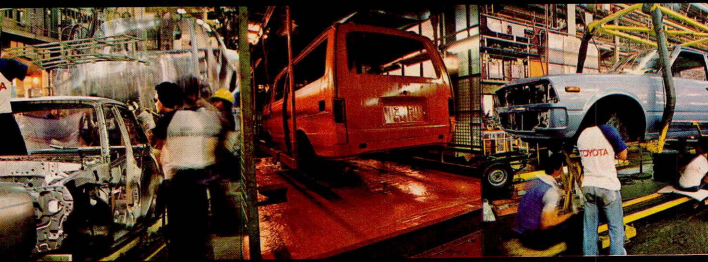
L-R: Corona on the trim line being subjected to gas brazing of roof and quarter panel; a Hi-Ace viewed right after treatment in primer EDP; and body drop of Toyota Corona.
