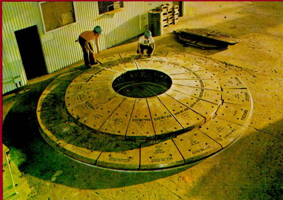
Top: Power shovel track pads for export. Bottom: Special alloy steel ball mill end liners for export.
