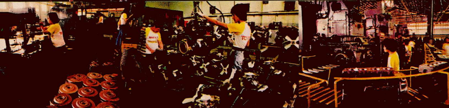
Top: L-R: Inspection of machine exhaust manifold, carburettor, and pistons, and machining line for cylinder wheels. Bottom: L-R: Flywheel balancing firing bench tests for 12R engines being carried out in background, and engines prepared for storage after testing and adjustments, and precision drilling of components.
