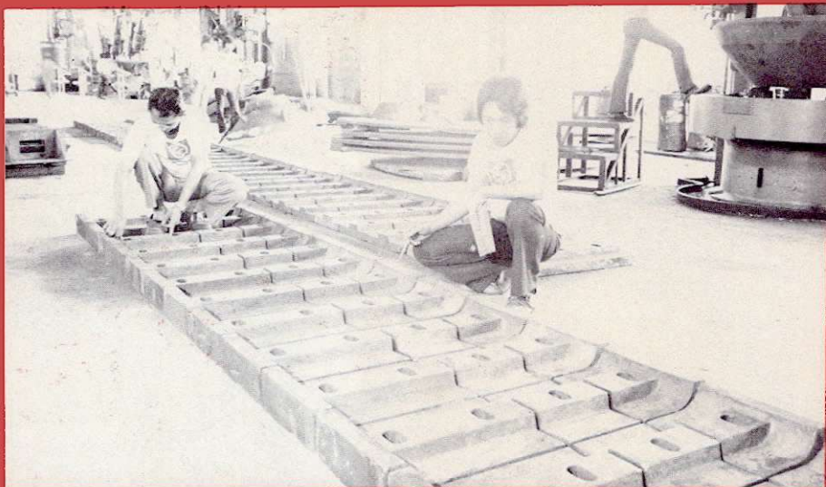
Ball Mill Shell liners made from ESCO alloy material for Thailand cement company.
