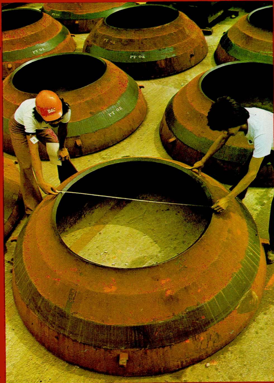
7-foot bowl and mantle liners for export to Bougainville copper mine.
