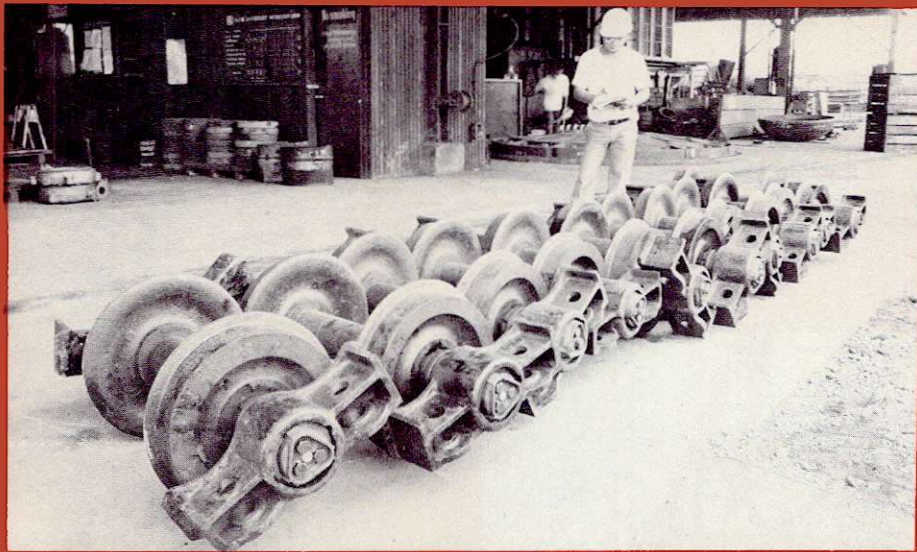
Mine car wheel and axle assemblies, EEI introduced the use of tapered roller
