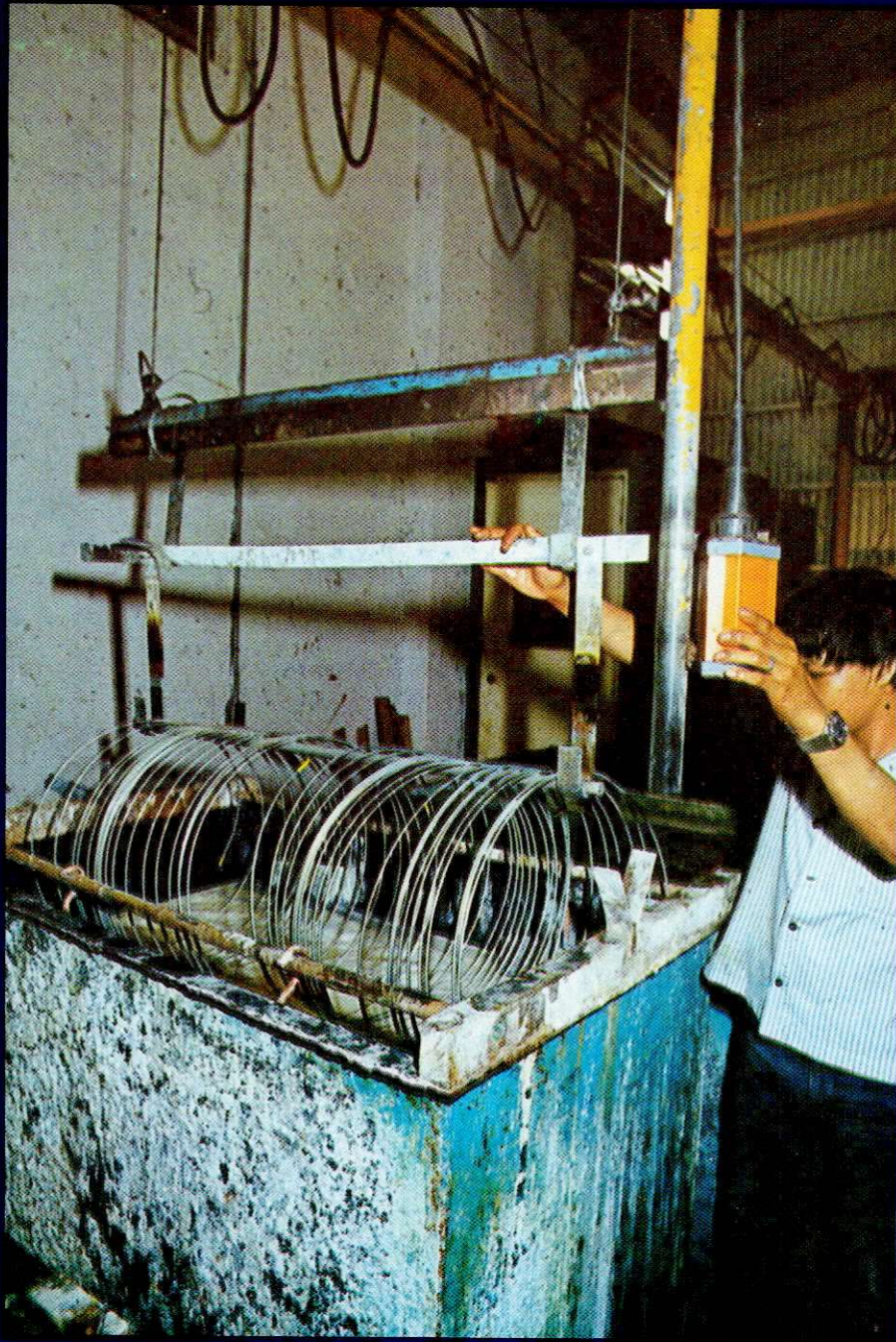
(Top) Corrosion resistance is enhanced by electrolytic zinc coating of bundyweld tubes. (Top right) The tubes are bent to serpentine wire fins for condenser assemblies. These are electric-resistance-welded to assure uniform adhesion while maintaining the desired physical and mechanical properties of the tubes and the finished condensers as a whole.
