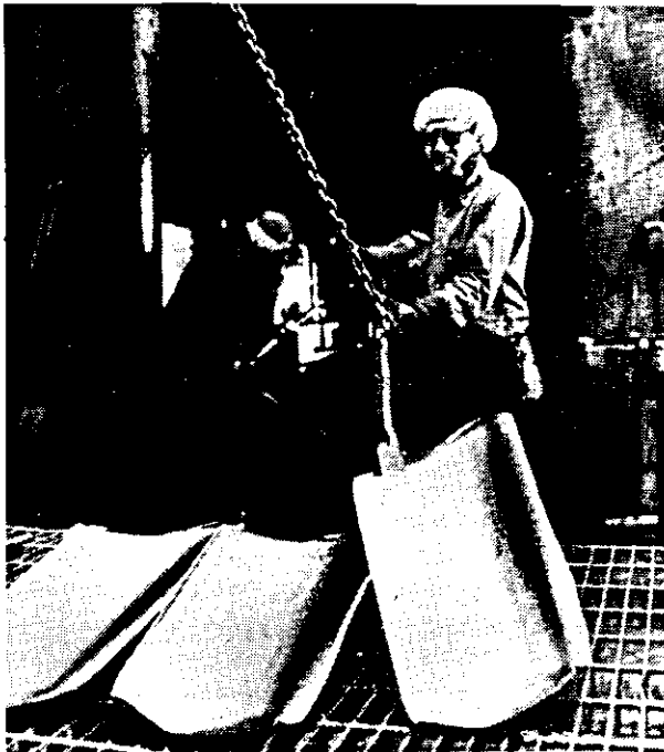
Westinghouse Electric Corporation forges large stainless steel vanes for use in electric generating stations.
