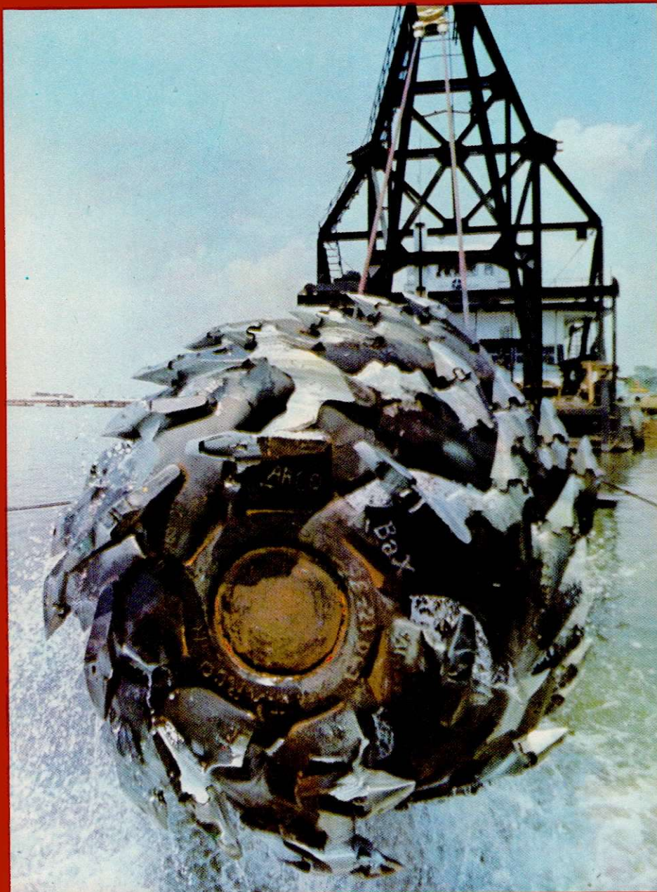
ESCO dredge cutter teeth used by Construction and Development Corp. of the Philippines.
