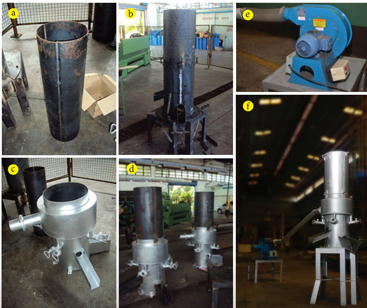
Fig. 2: Various stages of micro cupola fabrication: (a) shaft fabrication, (b) stand and other accessories, (c) tuyere and wind belt fabrication, (d) tuyere and wind belt assembly, (e) blower and accessories assembly, (f) painting and completion of assembly.
