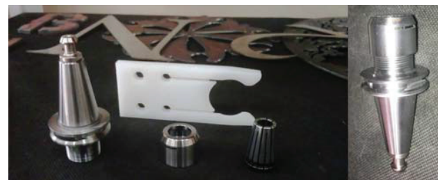
Fig. 8. ISO-20 tool holder system holder employed in the ATC system (see Fig. 8).
