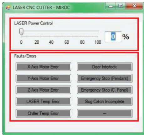
Fig. 11. GUI for the LASER power controller
