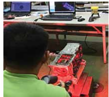
Figure 3. 3D scanning of an engine block.
