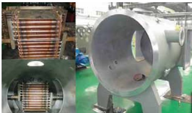
Figure 3. Picture (clockwise) shows the fabricated heat exchanger. Picture shows the finished vacuum vessel – outer shell. Picture shows the heat exchanger is installed at the rear of the vacuum vessel.
