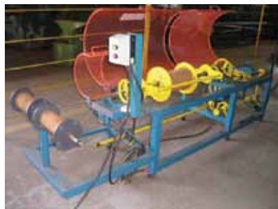
Figure 9. Twining machine with spooler
