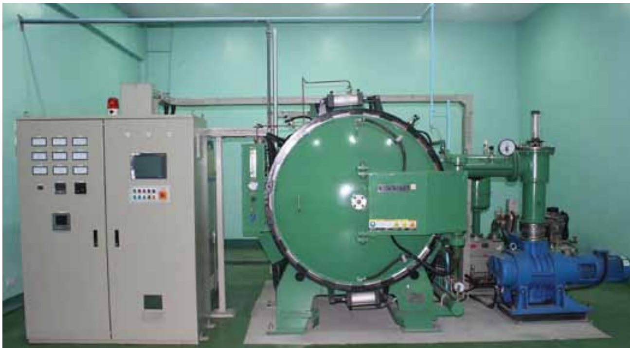
Figure 10. The Vacuum Gas Quench Heat Treatment Furnace.
