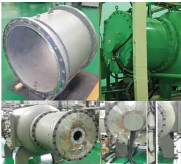
Figure 4. Images depicting the development/fabrication of motor fan vessel and installed at the back of the vacuum vessel.
