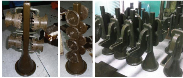
Figure 6. Clustering of wax pattern
