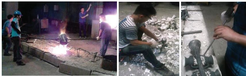
Figure 8. Melting and removal of ceramic shell
