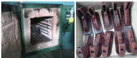
Figure 10. Stress relieving of some cast parts
