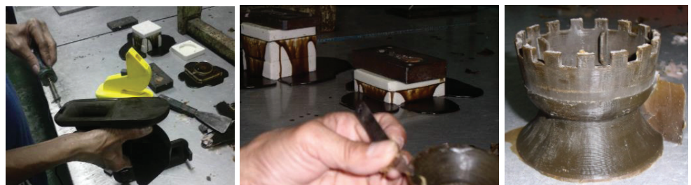
Figure 5. Repairing of wax pattern
