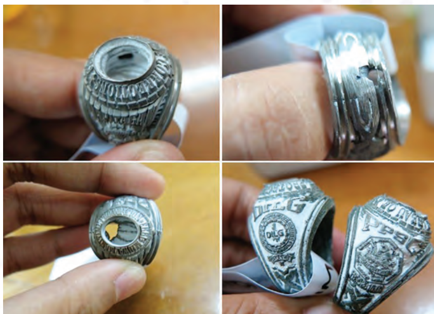
Figure 2. Common casting defects on cast emblem rings
