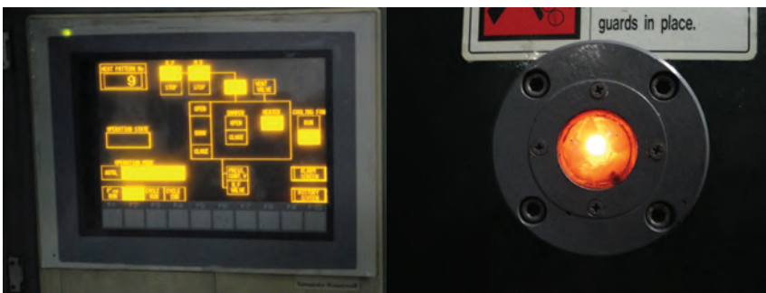
Figures 9 and 10. Touch screen control panel showing the status of the systems of vacuum furnace. Peeking through the sight glass shows glowing inside the chamber at elevated temperature.
