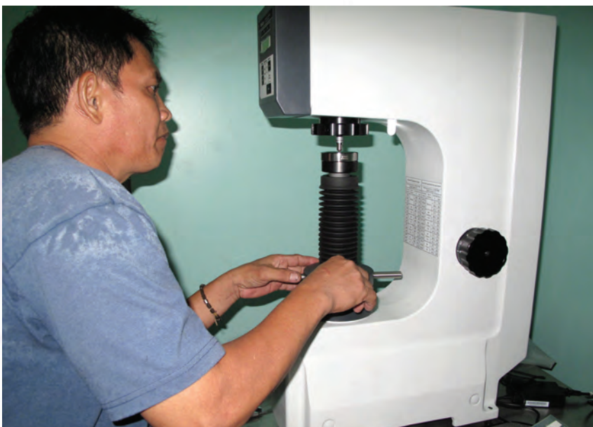
Figure 11. Heat Treatment personnel conducting hardness testing on heat treated samples to confirm transformation of microstructure and achieving desired hardness.
