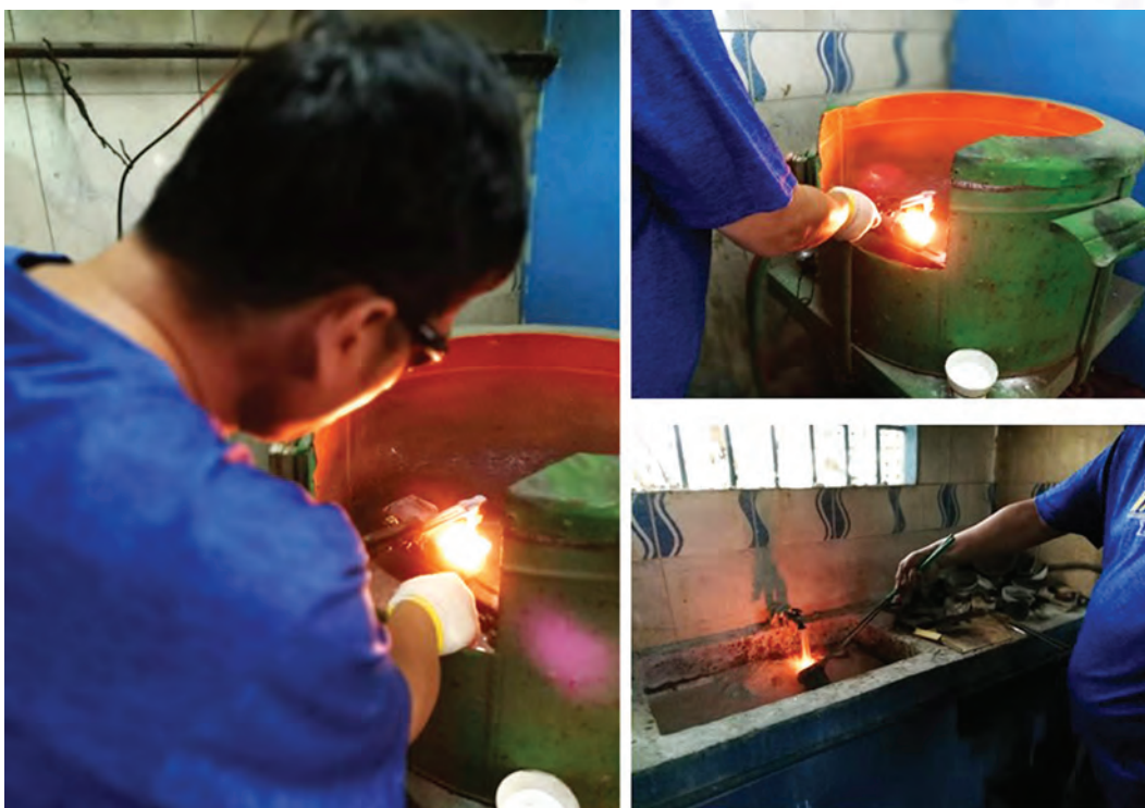
Figure 7. Casting and burnout
