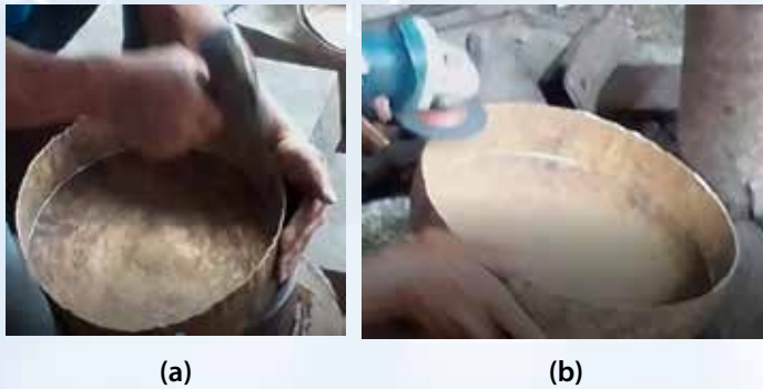
FIGURE 4. Cornering (a) and grinding (b) results to the basic gong
