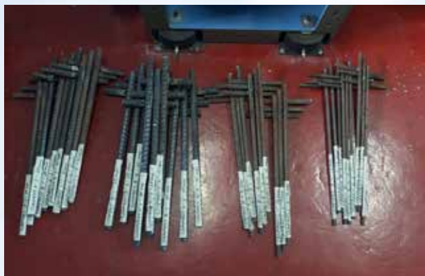
Figure 3. Welded samples for testing
