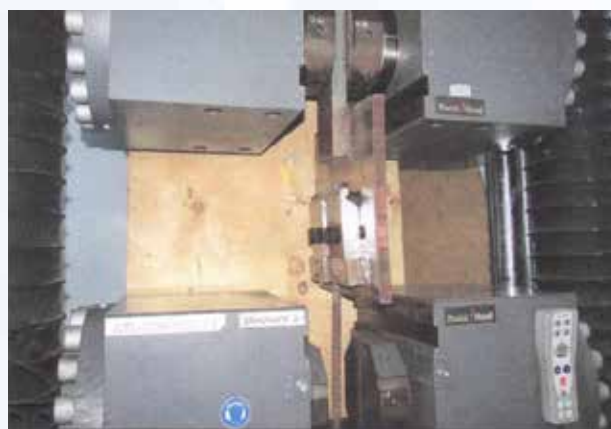
Figure 4. Test setup for the shear test of rebar wire mesh using the fabricated jig
