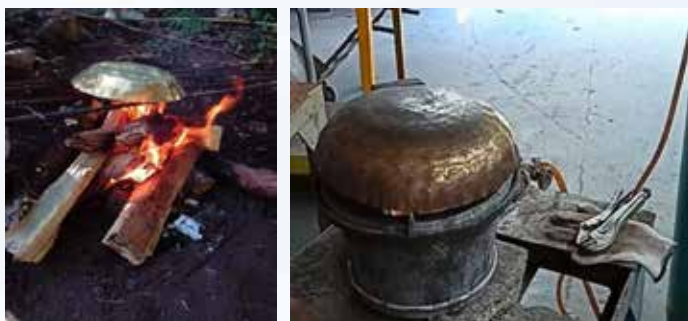
FIGURE 2. Heating to remove stress due to hammering, a) using wood and b) using LPG as fuel
