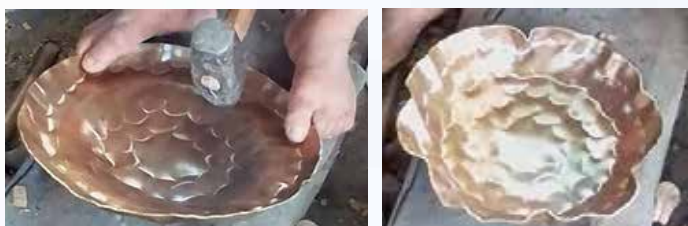
FIGURE 1. The material after the third (a) and the fourth (b) round of hammering
