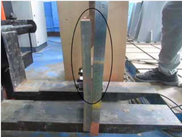
Figure 5. Photo showing permanent deformation after testing 25mm Ø
