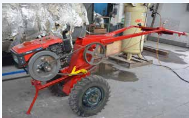
Figure 9. The developed hand tractor with gear transmission prototype
