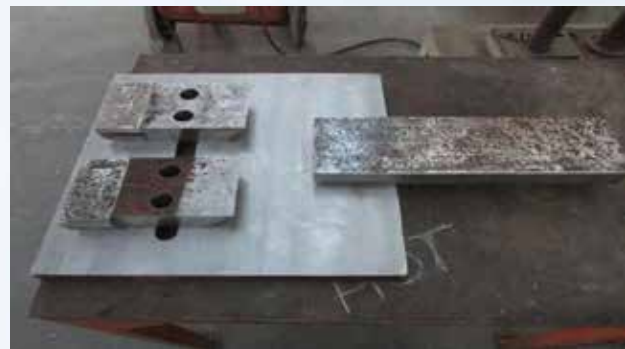
Figure 2. Body of the test jig after machining to designed dimension
