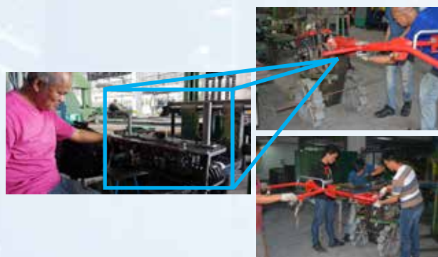
Figure 4. Integrating the gear transmission system to a hand tractor
