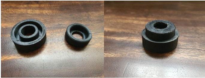
Figure 6. (left) Fit check for top/bottom cap and core interface; (right) fit check for top/bottom cap and core interface – mated
