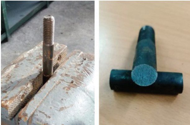
Figure 9. A flat fracture surface (right) indicative of brittleness was obtained by smashing with hammer while one end is clamped (left).
