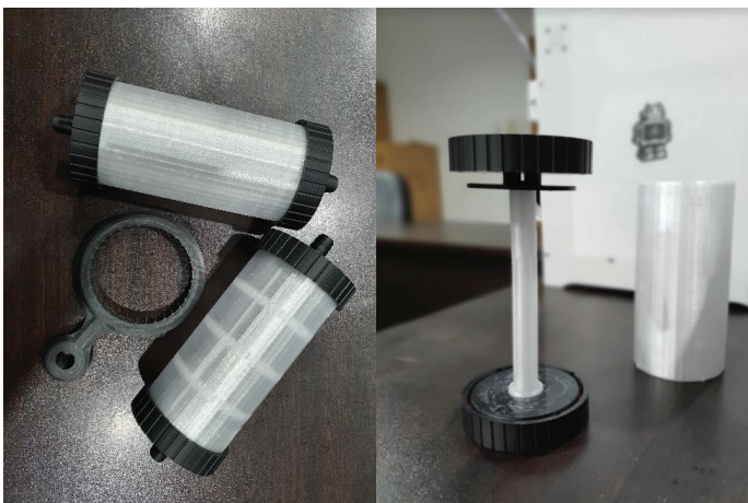
Figure 9. (a) full assemblies of the final prototype (b) internal assembly components of the final prototype showing the core and core barrier
