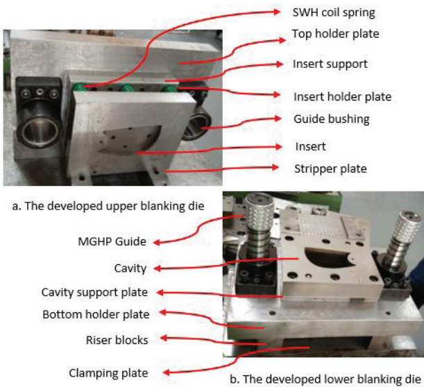
Figure 11. The developed blanking die for propeller's blade
