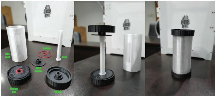
Figure 7. (left) Individual printed components, (middle) internal assembly, and (right) the full assembly
