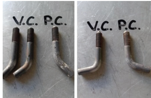
Figure 10. Samples did not fracture when manually tested for static bend test using G.I. pipe (left) and impact bend test by smashing with hammer. Vacuum carburized bolts were labeled as VC, while pack carburized bolts as PC.
