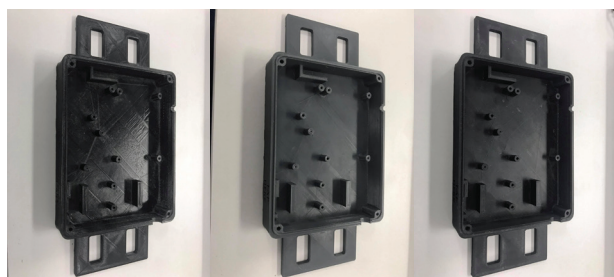
Figure 5. 3D printed enclosures made from (a) PC, (b) CPE and (c) Tough PLA.
