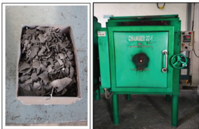
Figure 2. Sample were packed in a stainless steel box filled with charcoal and barium carbonate is added as energizer (left). The box is loaded inside the electric furnace (right).
