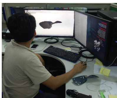
b. Exporting point cloud to NX CAD software for 3D Modelling
