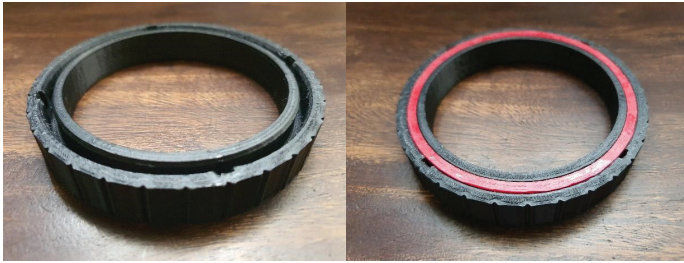
Figure 5. (left) Fit check portion for the top/bottom cap and (right) fit check of O-ring and top/bottom cap
