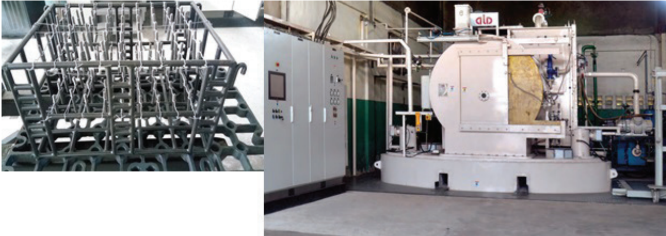
Figure 4. Samples were tied with G.I. wires and arranged with adequate space for subsequent oil quenching (left). MIRDC vacuum carburizing furnace with hot zone dimension of 600x750x1000mm.
