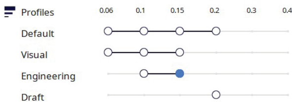
Figure 2. Available profiles for Tough PLA from the software, Cura.
