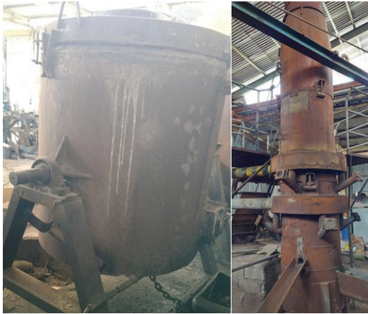
Fig. 3. A. New Crucible Furnace; B. Modified Cupola Furnace
