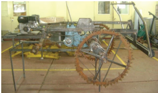
Fig. 1. Vietnamese Transmission Gearbox Used in the Transplanter
