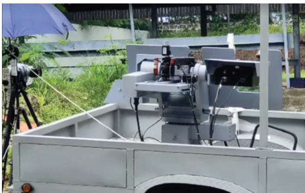
Fig 2. High-Speed Camera Setup During Live-Fire Testing of BUHAWI
