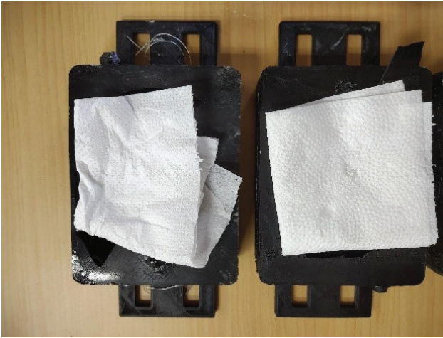
Fig. 8. Photos of the enclosure after the liquid ingress test.
