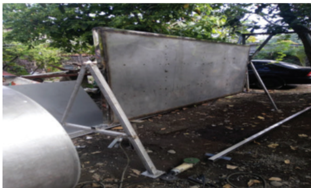
Fig. 2. Completed Stainless-Steel Steam Dryer
