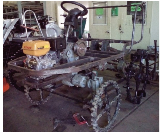
Fig. 3. Localized Vietnamese Transmission Gearbox Used in the Second Prototyped.
