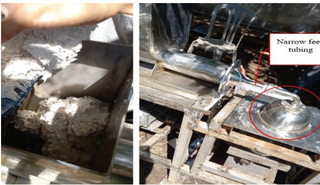
Fig. 7. (L) Screw Feeder and (R) Molding Plates of Molding Machine Showing the Narrow Feeding Tube
