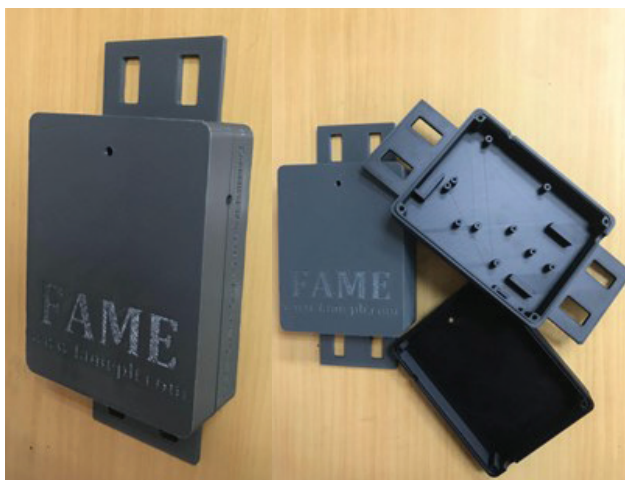
Fig. 7. Actual photos of the 3D-printed transponder enclosure assembled and disassembled.
