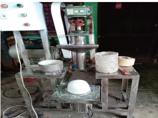
Fig. 8. Final Molder Design
