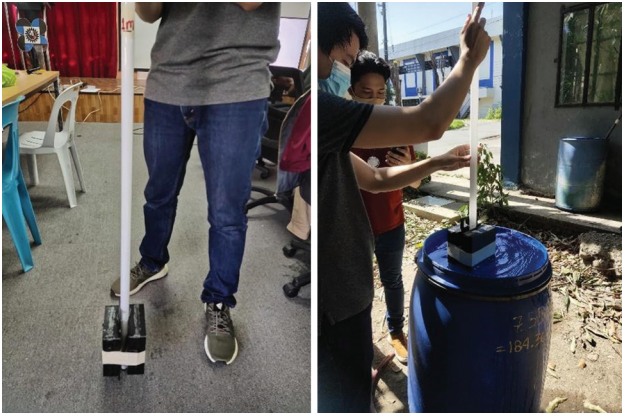
Fig. 2. (L) Casings Taped Together for a (R) One-Meter Liquid Ingress Test Done in a Water Drum.
