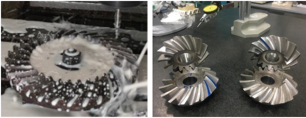
Fig. 7. Cutting the Designed Spiral Bevel Gear on a 5-Axis Machining Center
