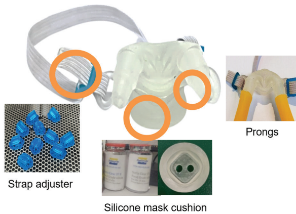
Fig. 5. 3D Printed Nasal Mask Assembly
