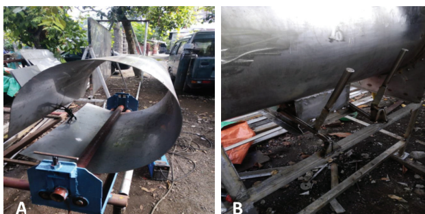
Fig. 3. (A) Rolling of Mixer Body and (B) Completed Clay Dough Mixer
