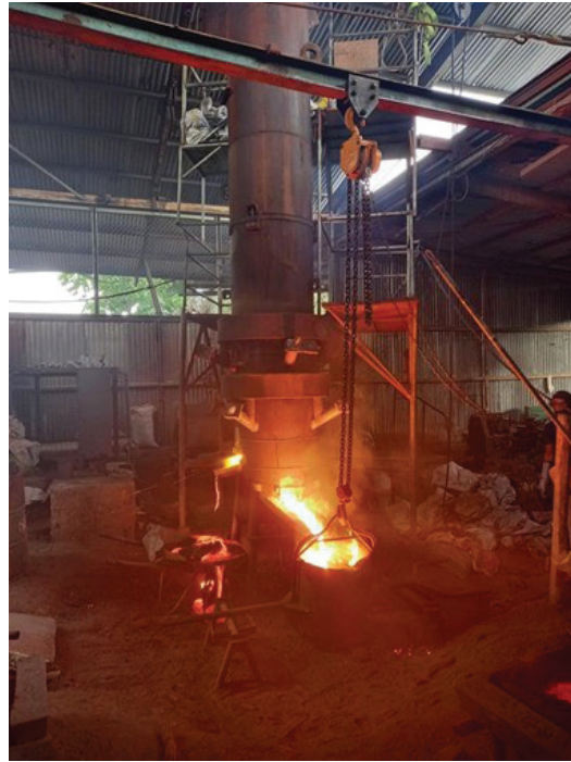
Fig. 4. Final Testing of the Cupola on November 2021
