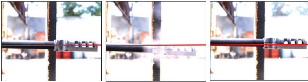
Fig. 9 Barrel Deflection Without Recoil Compensator Caught Using a High-Speed Camera at Burst Fire of Two Bullets
