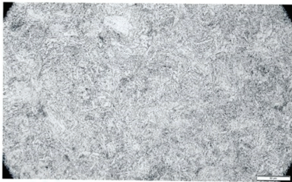
Photomicrograph of Parameter 3 Etched with Nital, 500x magnification
