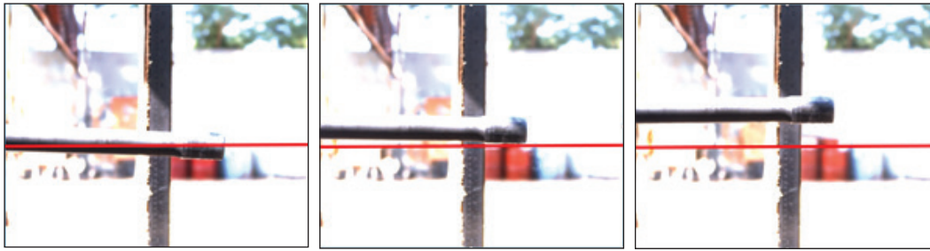
Fig. 4 Barrel Deflection Without Recoil Compensator Caught Using a High-Speed Camera at Burst Fire of Two Bullets
