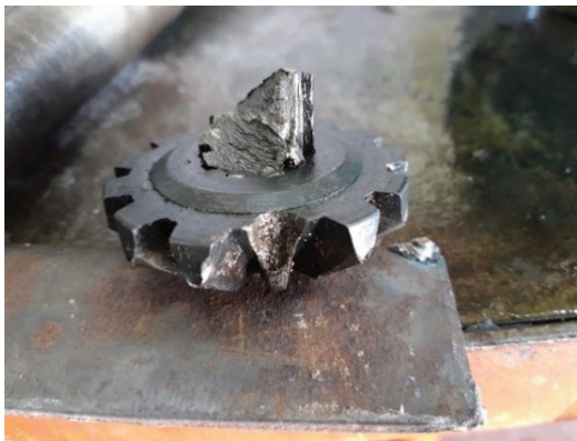
Fig. 6. Damage on Spindle Drive
