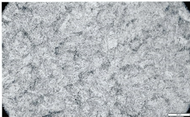
Photomicrograph of Parameter 4 Etched with Nital, 500x magnification
