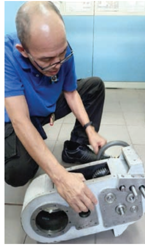
Fig. 5. Testing of the improved gear shifting mechanism
