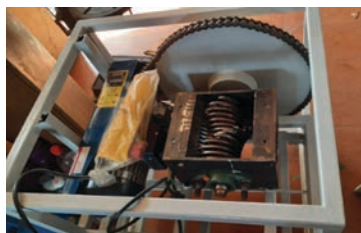
Fig. 4. Fabricated shredder machine in meter and ECU assembly
