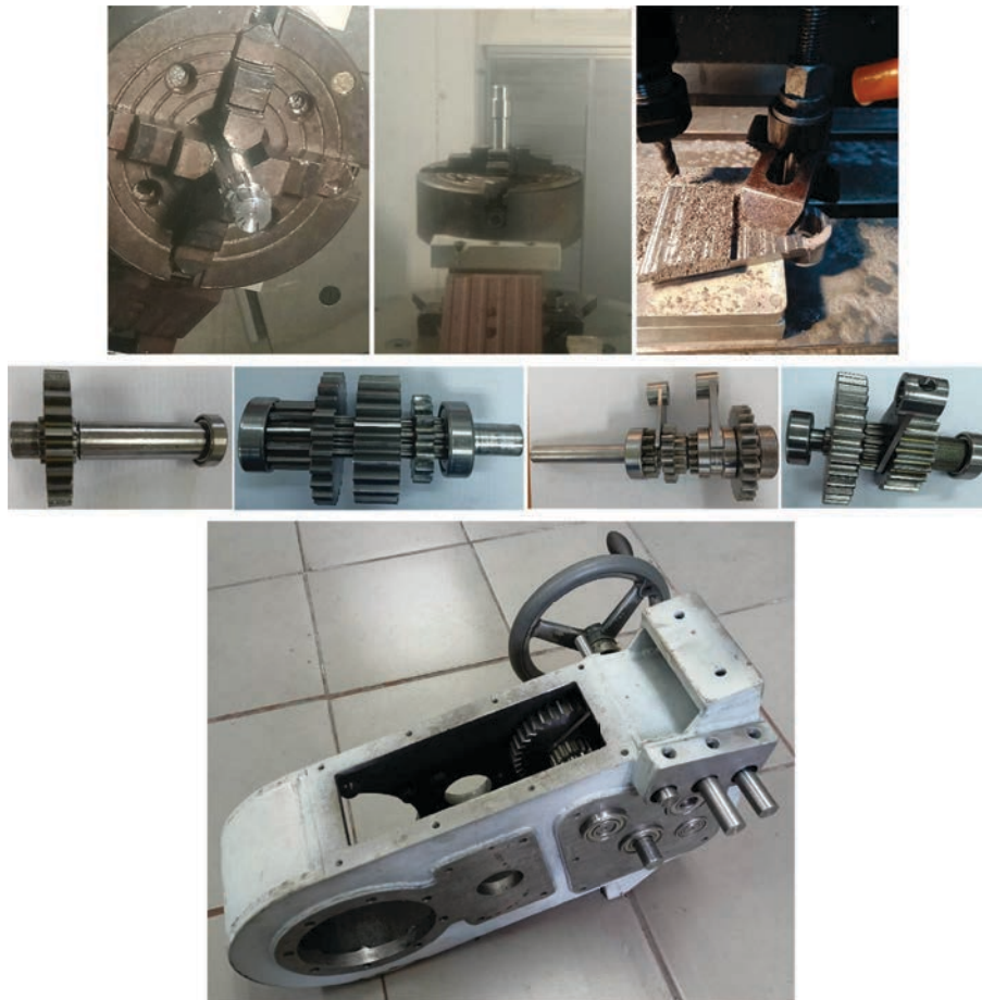
Fig. 4. Fabrication and assembly of the gear shifter
