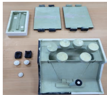
Fig. 16. The assembled 3D printed pattern of the rear lid ready for molding
