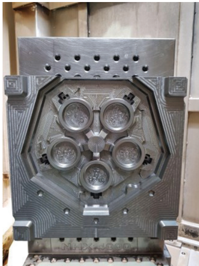
Fig. 5. CNC machined pattern using a horizontal 3-axis milling machine
