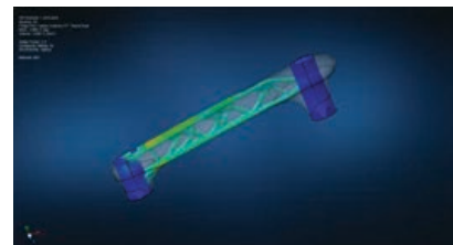
Fig. 6. Connecting Link Topology Optimization
