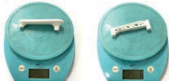
Fig. 11. Weight comparison between unoptimized (L) and optimized (R) connecting link
