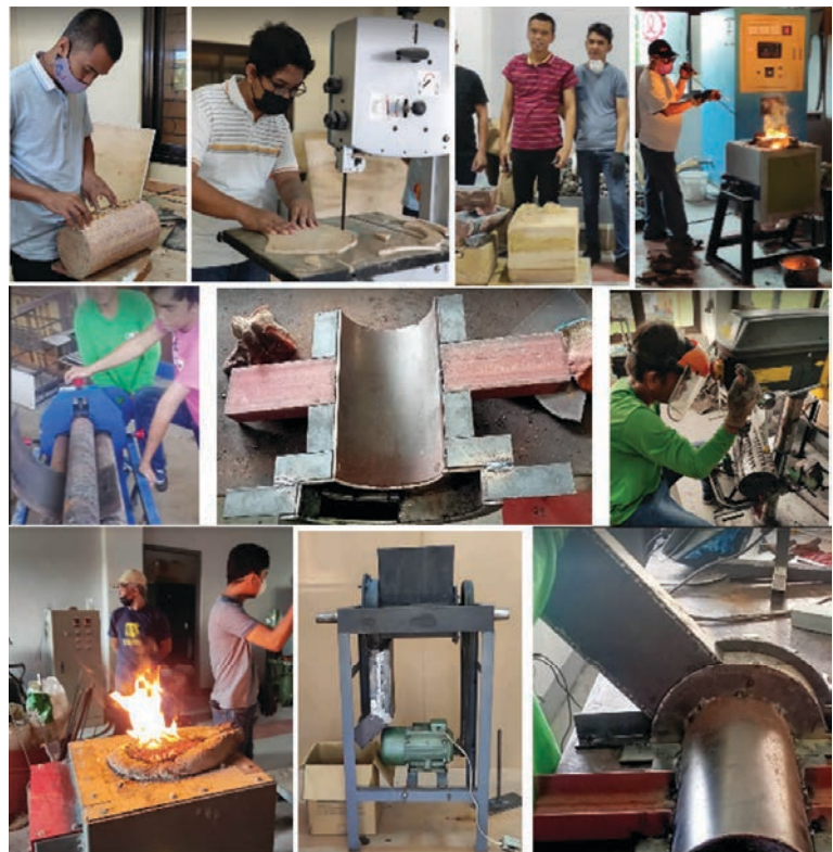
Fig. 5. Fabrication of the coconut coir and coco peat extraction device.
