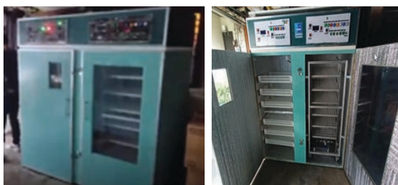
Fig. 3. Actual System Device of the Augmented Poultry Egg Hatchery
