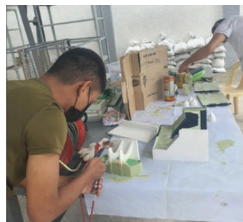
Fig. 15. Application of primer in order to improve abrasion/wear and chemical resistance of the 3D printed pattern
