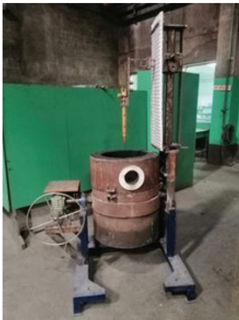
Fig. 4. Prototype of final design of BOF and oxygen lance
