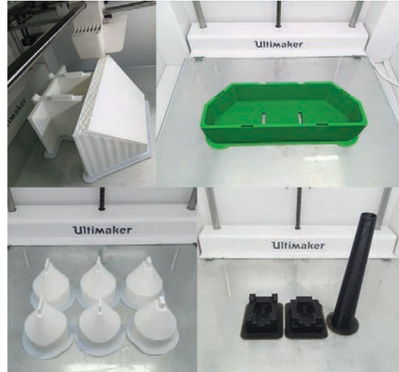
Fig. 13. 3D printing of the pattern components of the rear lid
