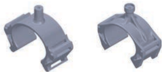
Fig. 7. Model from MSC Apex (left) and finalized model from Solidworks (right) of the drone clamp
