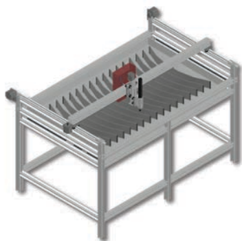
Fig. 1. Isometric view of the CNC Plasma Cutter
