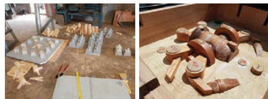
Fig. 1. Conventionally fabricated wooden patterns
