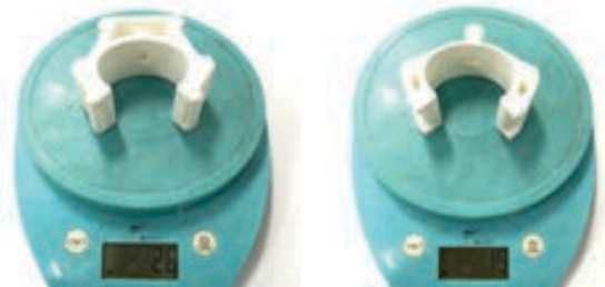
Fig. 12. Weight comparison between unoptimized (L) and optimized (R) drone clamp
