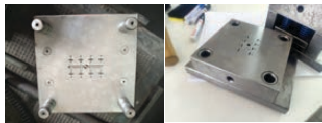
Fig. 3. Core and Cavity molds designed, fabricated, and used for local production of dosimeter security locks
