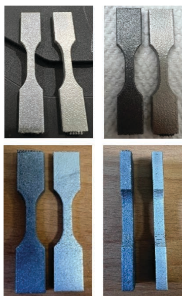
Fig. 14. Photographs of electropolished AM aluminum samples: unpolished (left), and electropolished (right)
