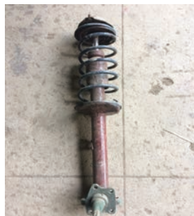
Fig. 1. Pre-assembled coil spring suspension
