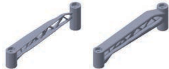
Fig. 8. Model from MSC Apex (left) and finalized model from Solidworks (right) of the connecting link
