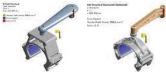
Fig. 3. FEA Simulation Load, Condition and Constraint
