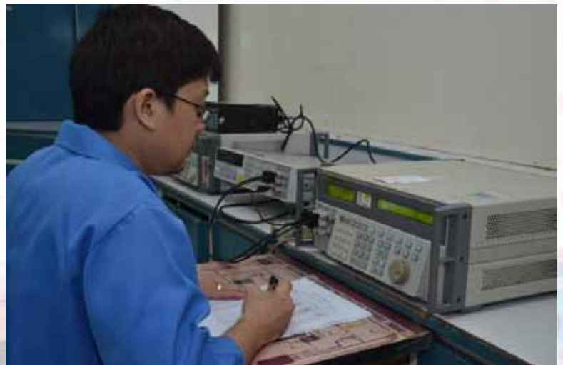
Calibration of electrical calibrator using a standard DMM
