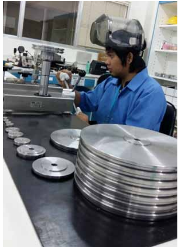
Calibration of pressure gauge using dead weight tester
