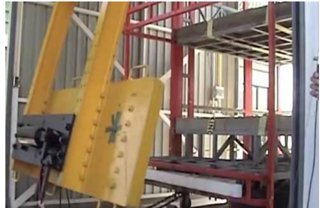
Transport Body Impact Tester
