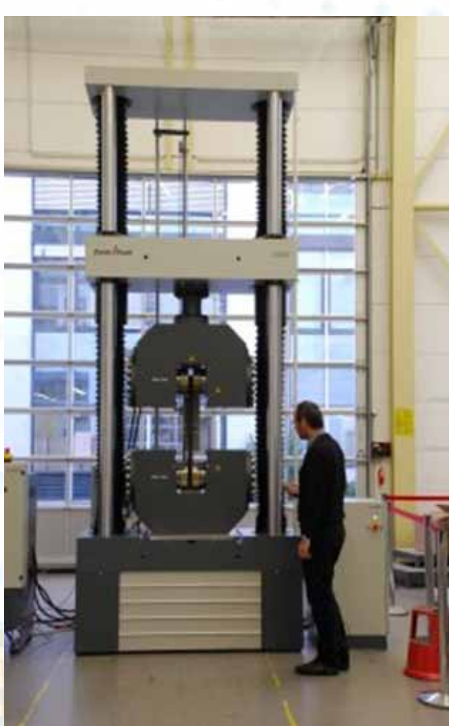
200T Universal Testing Machine
