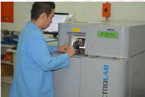
Optical Emission Spectrometer, OES – Spark (Ferrous & Nonferrous materials - Cu, Al & Sn)
