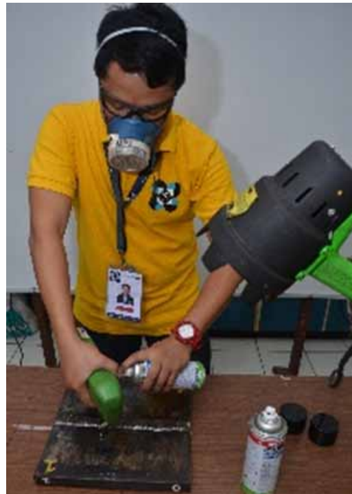
Magnetic Particle Inspection
