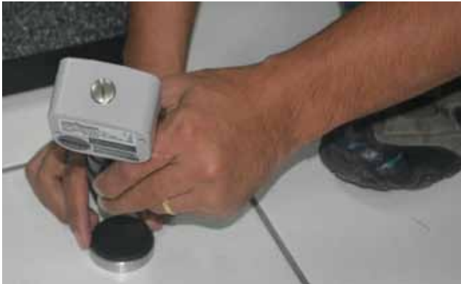
Durometer (Shore A)
