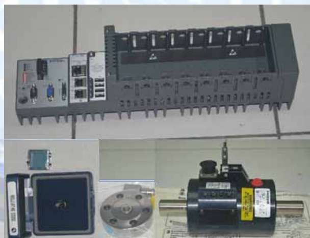
Data Recorder/Analyzer with Accelerometer, Load Cell and Torque Sensor
