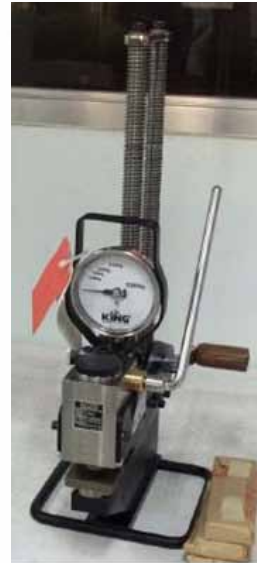
Brinell Hardness Tester
