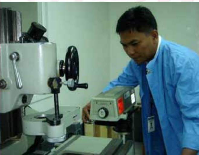
Calibration of length standards, glass scale, metal rules using HP Laser and universal measuring machine
