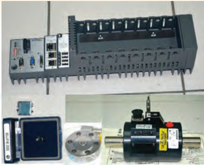
Data Recorder/Analyzer with Accelerometer, Load Cell and Torque Sensor
