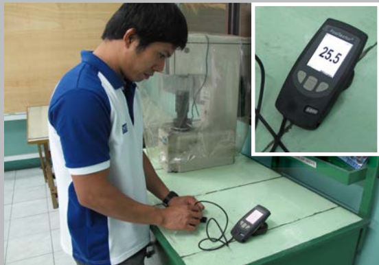
Thickness testing on the anodized products.
