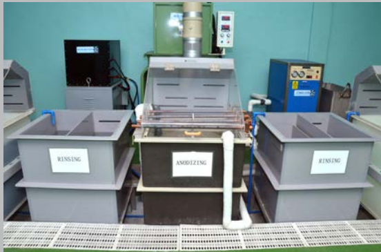
Rectifier is used as direct current source to operate any plating or anodizing system.
