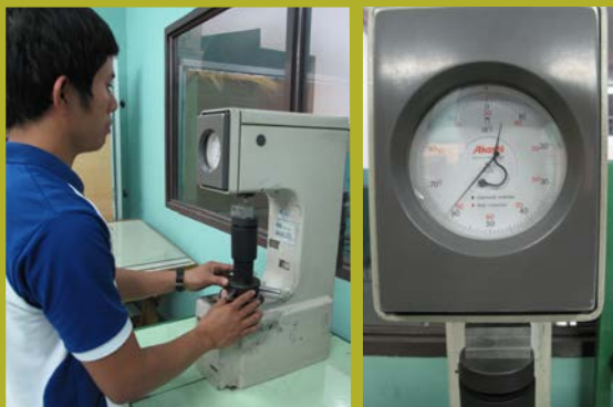
Hardness testing on heat treated samples to confirm change in physical property.
