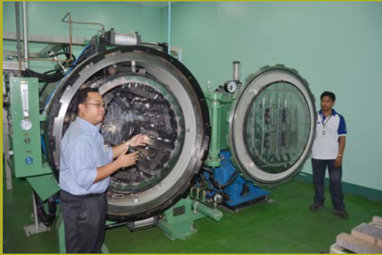
Discussion of vacuum heat treatment furnace operations
