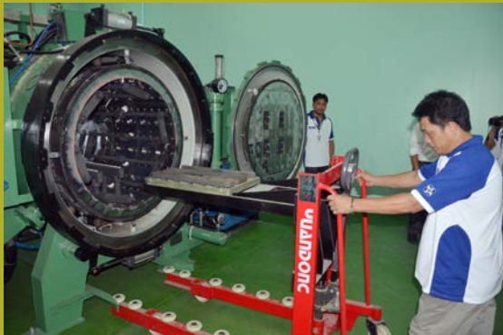
Charging of D2 Tool Steels in the VHT Furnace for hardening heat treatment.
