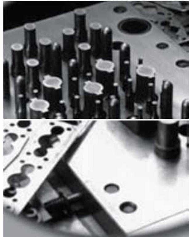
Figure 16b. Piercing/Embossing and Progressive dies
