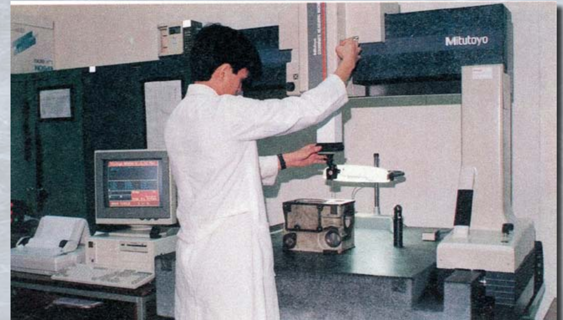
A Mitutoyo Coordinate Measuring Machine, one of the GTZ-acquired precision equipment for the MIRDC Metrology Laboratory
