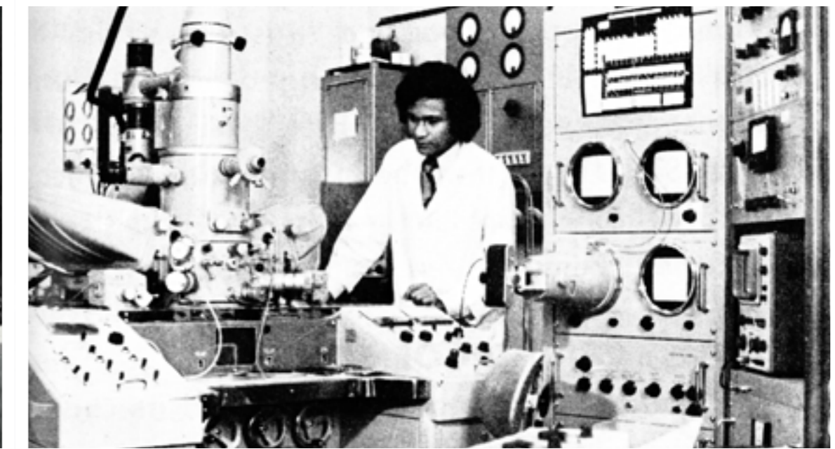
Marcelo B. Villanueva operates the microprobe analyzer, a sophisticated apparatus in electron microscopy | 1973
