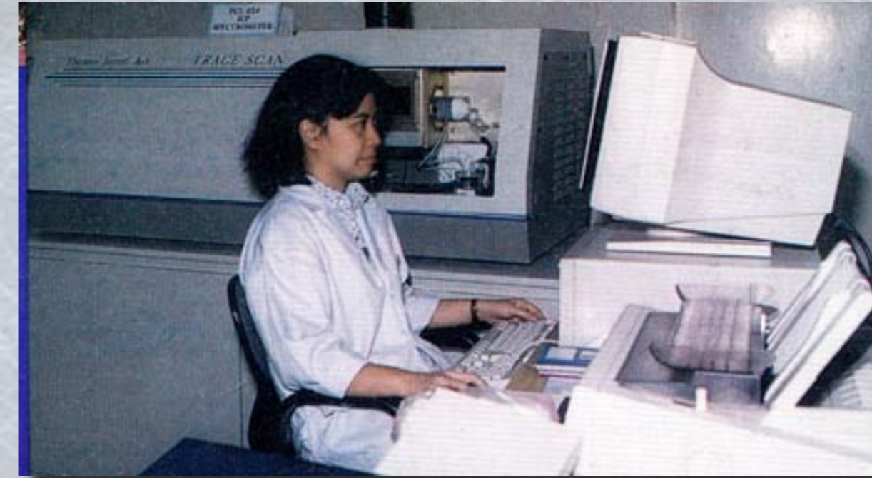
Induction Coupled Plasma (ICP) Analyzer traces minor and major components of metal alloys
