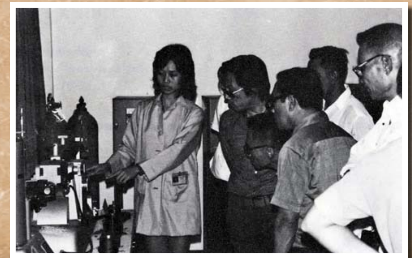
Engr. Moreno demonstrates the use of a universal sand strength tester | 1973
