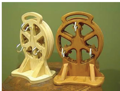
Fig. 7. Portable three strand gear type hook rope machine
